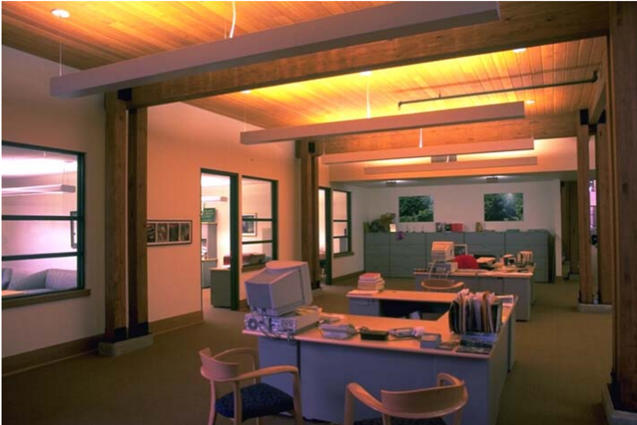
Figure 4 Minimize direct glare with indirect lighting.
