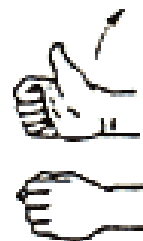
Hold load and raise boom
