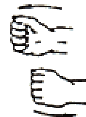
Track motions turning caterpillar
