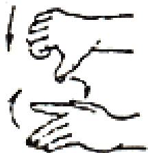
Raise load and lower boom
