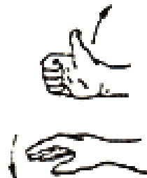
Lower load and raise boom
