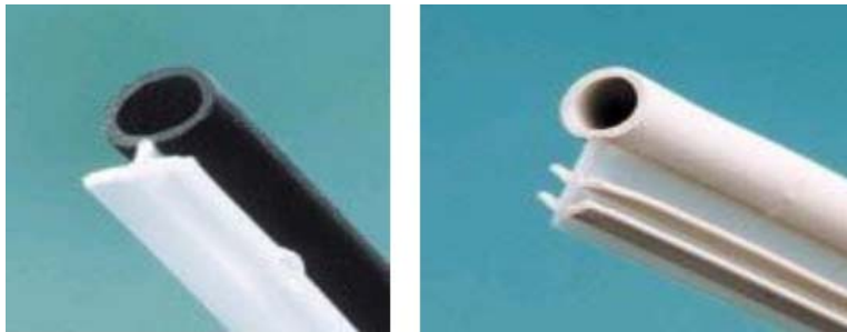
Figure 9. Left: Bulb weatherstrip with a rigid backer for threading into a slot which has been extruded into an aluminum or PVC sash or frame. Right: Bulb weatherstrip equipped with a “double-dart” designed to be permanently pressed into a slot cut along the edge of a wood window frame or sash. These weatherstrips are extruded from vinyl, TPEs (thermoplastic elastomers), PVC, silicon, polypropylene and jacketed foams.
