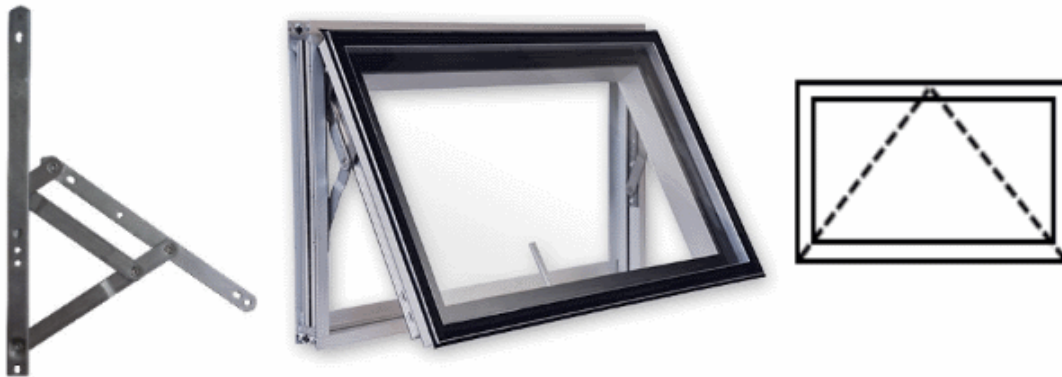
Figure 6. Project out vent (center). At left is the scissors hinge that is installed in the jambs (sides), yet at right, the convention for indicating operation with dotted lines formed into a V, point at the theoretical hinge location at the top, as if the hinges were butt hinges as used on a typical door.
