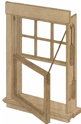
Figure 5. Double hung window showing rope, pulley and counterweight
