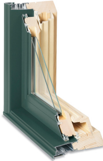
Figure 14. Aluminum clad wood window. Wood (at right) is exposed to the interior while protected on the exterior by aluminum cladding. This design, sometimes using a PVC cladding in lieu of aluminum, is commonly used in residential construction.
