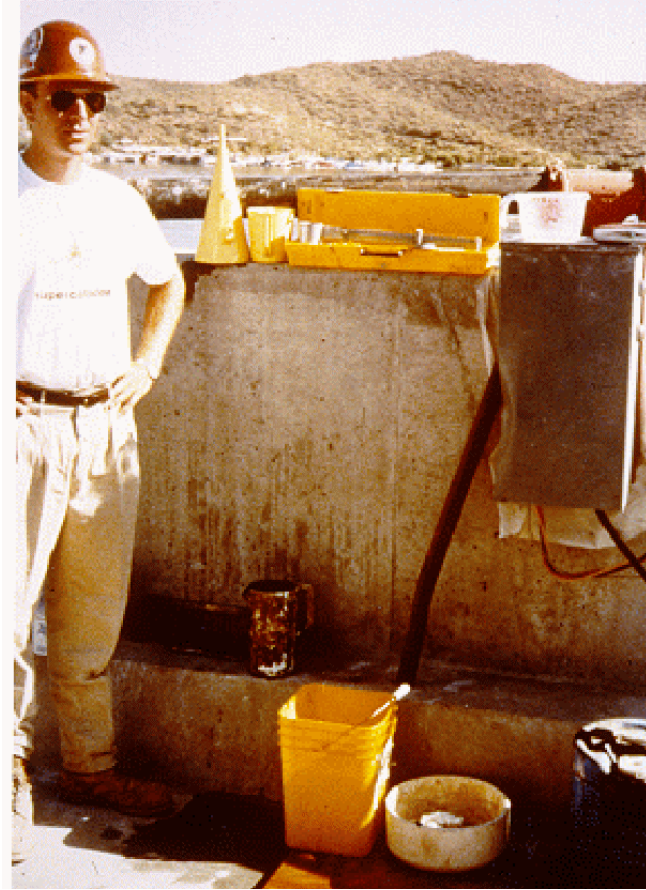
Figure 8-8. Baroid Mud Balance Test.
