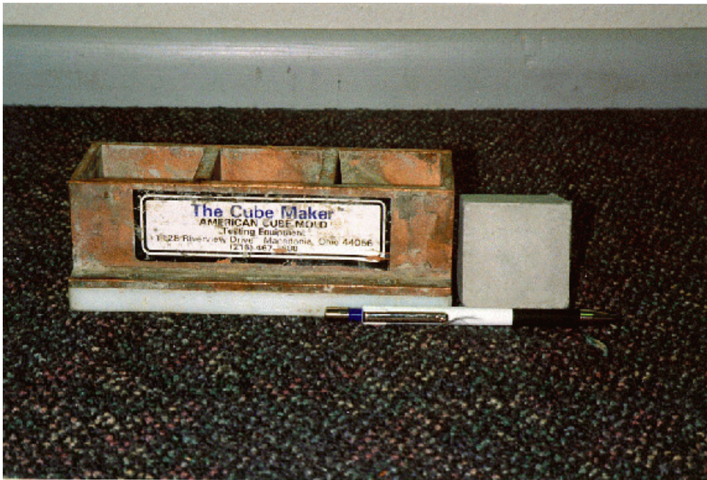
Figure 8-7. Grout Cubes for Compressive Strength Testing.
