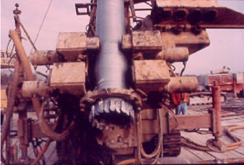
Figure 4-5. Casing with Heavy Duty Casing Crown.
