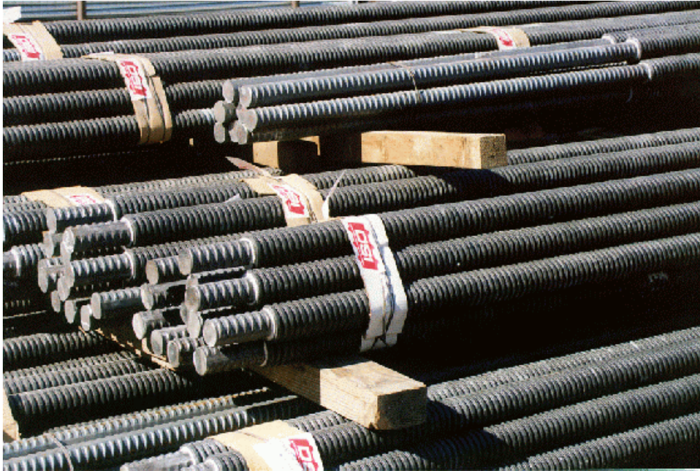
Figure 8-4. Double Corrosion Protected (Encapsulated) Reinforcing Steel.
