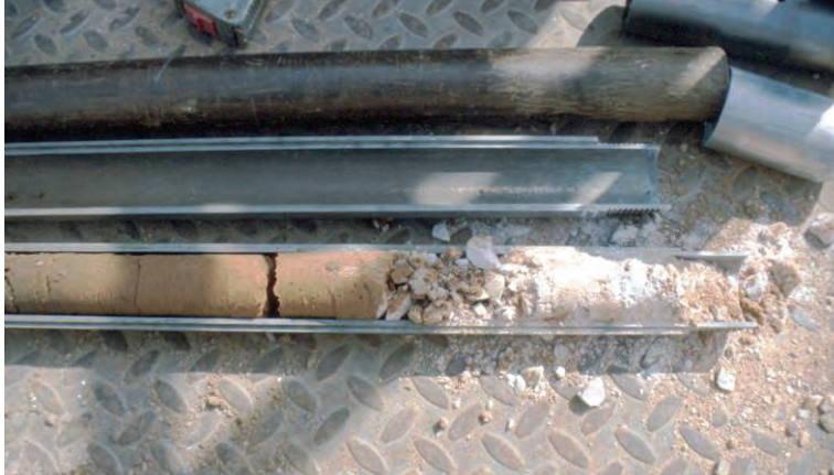
Figure 3-2 Split-Spoon Sampler for Determination of Soil Stratigraphy
