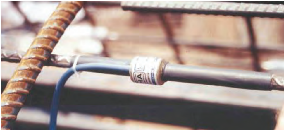
Figure 17-50 Vibrating Wire Type Strain Gauge
