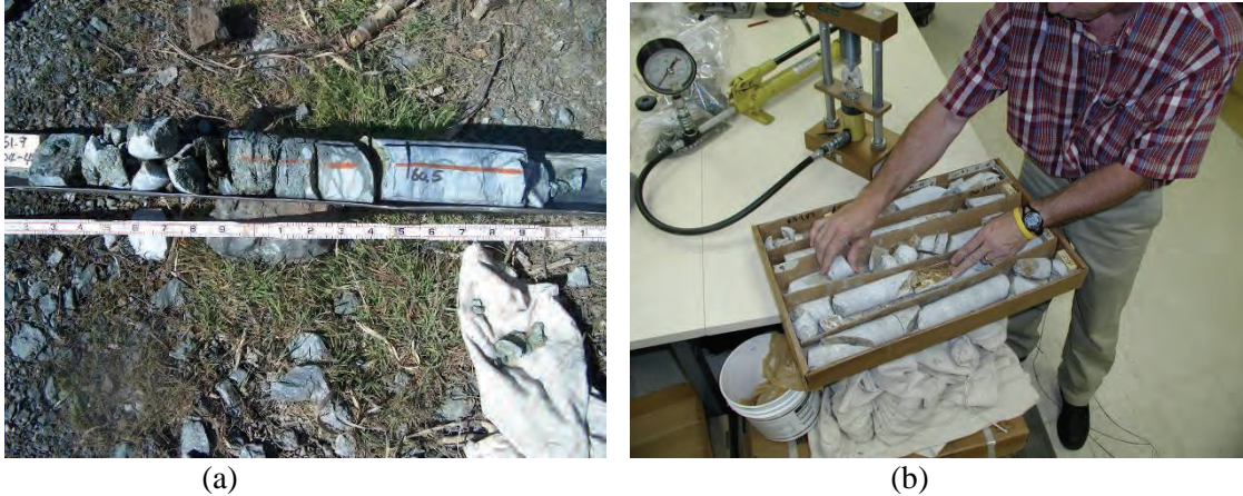
Figure 2-6 Field Photography of (a) Rock Core in the Sampler; and (b) Rock Core Stored in Boxes
