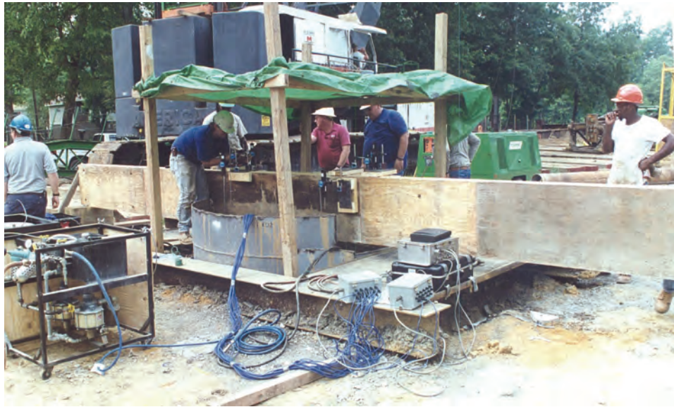
Figure 17-3 Instrumented Research Load Test
