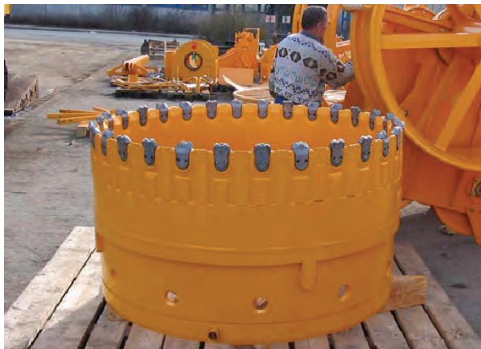
Figure 6-9 Cutting Shoe for Segmental Casing
