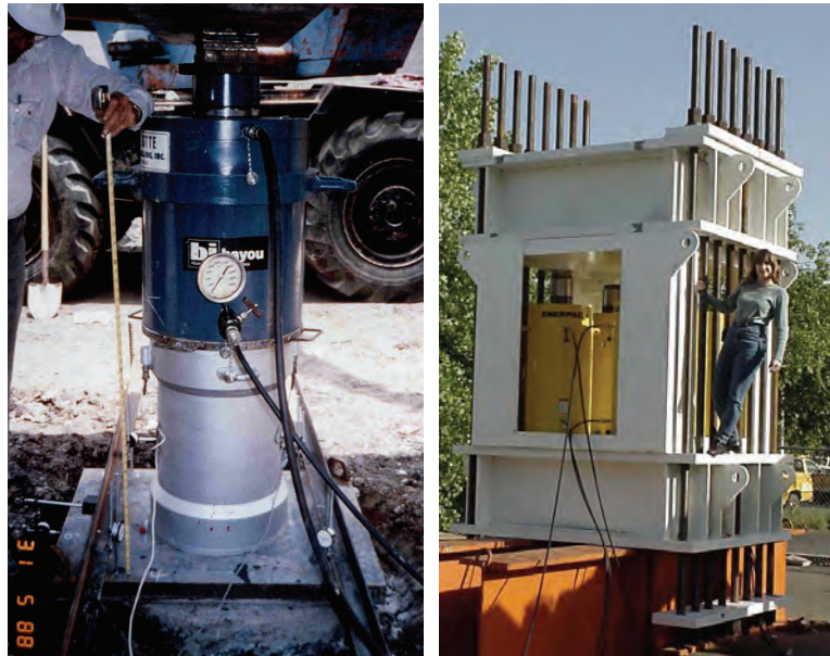
Figure 17-45 Hydraulic Jacks for Static Load Tests
