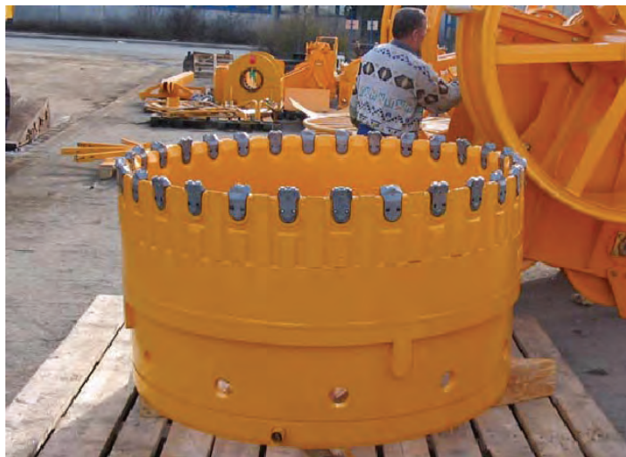
Figure 6-9 Cutting Shoe for Segmental Casing
