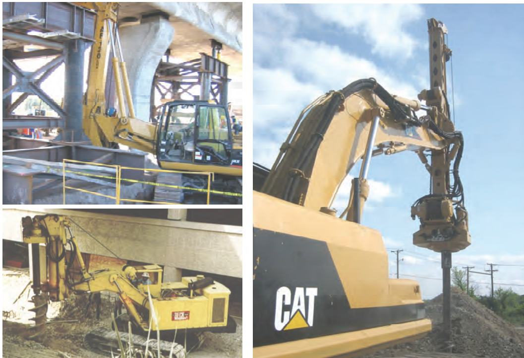
Figure 5-7 Excavator Mounted Drilling Machines for Restricted Overhead Conditions
