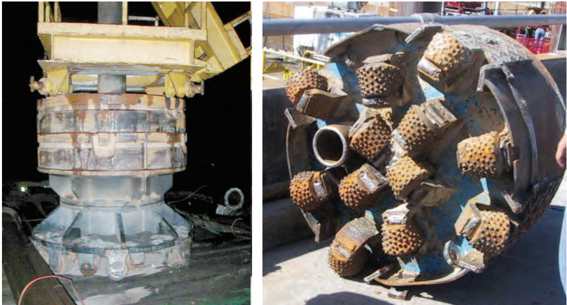
Figure 5-11 Reverse Circulation Cutting Heads for Top-Drive Drill
