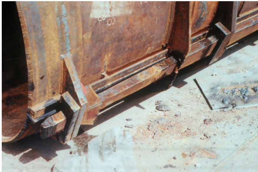
Figure 6-12 Locking Mechanism for a Removable Casing
