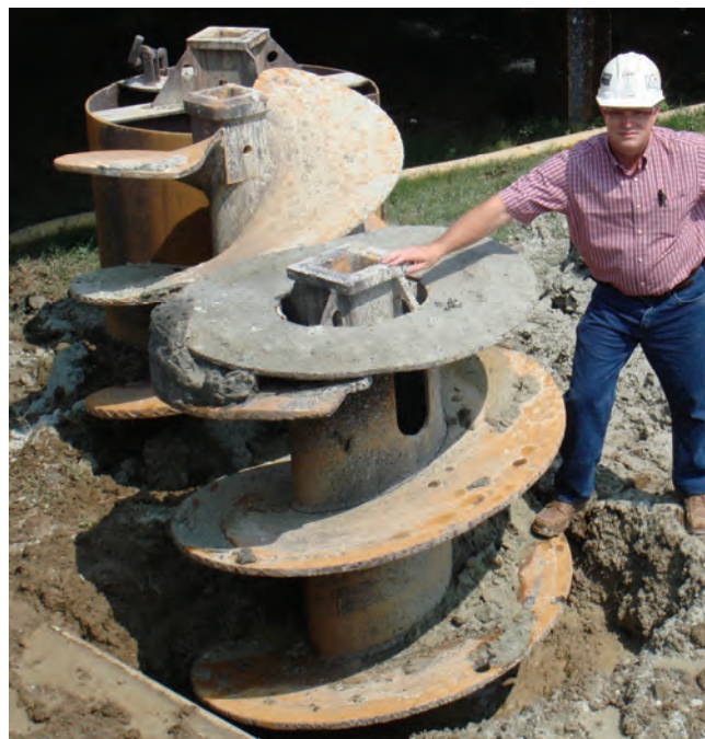
Figure 5-18 Auger with Slurry Bypass
