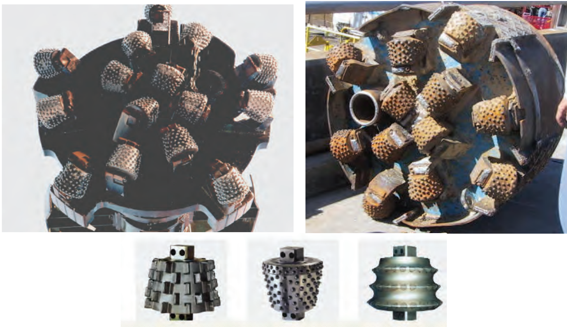
Figure 5-26 Full-Faced Rotary Cutters
