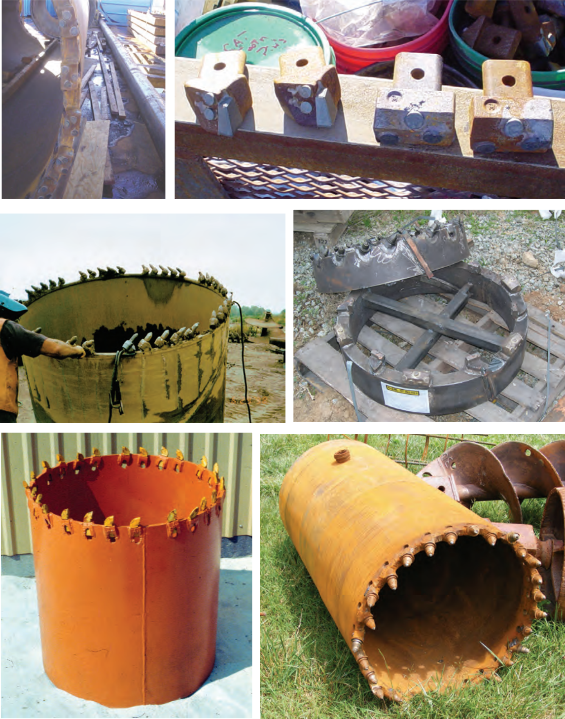
Figure 5-23 Single Wall Core Barrels
