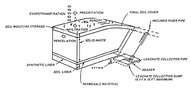
Figure 5-1. Cross Section of a Chemical Waste Landfill with Leachate Collection
