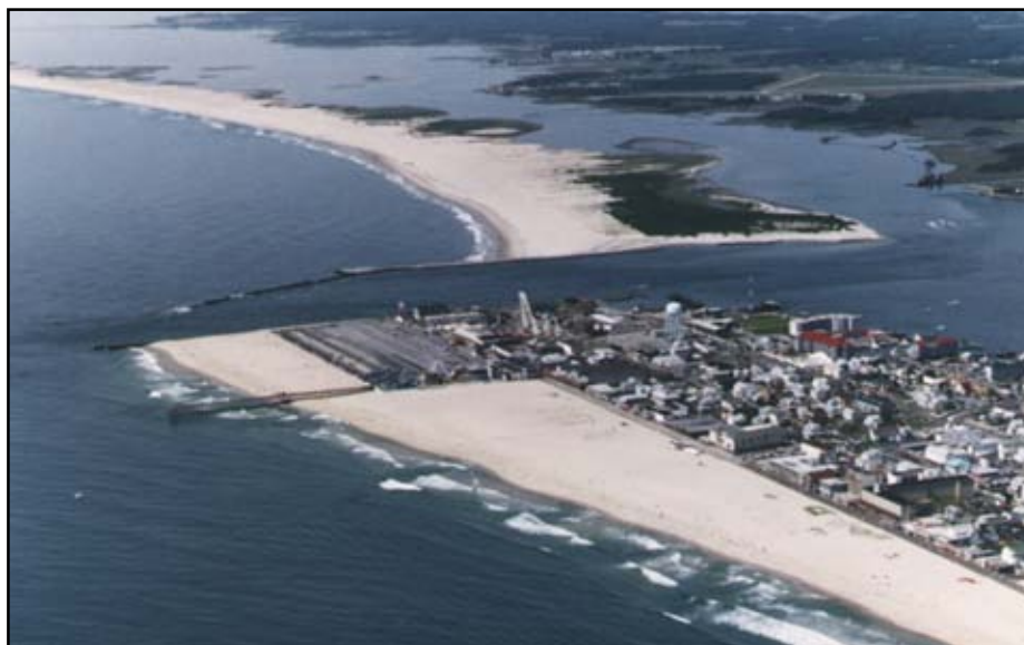
Figure 7-45 Ocean City Inlet, Maryland, was opened by a hurricane in 1933 and stabilized by jetties in 1934–35. Note extreme shoreline offset and downdrift erosion resulting from inlet stabilization. 1992 photograph.
