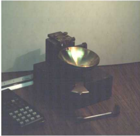
Figure 7-3. Liquid Limit Test by (a) Manual Casagrande Cup Device; (b) Electric Fall Cone.
