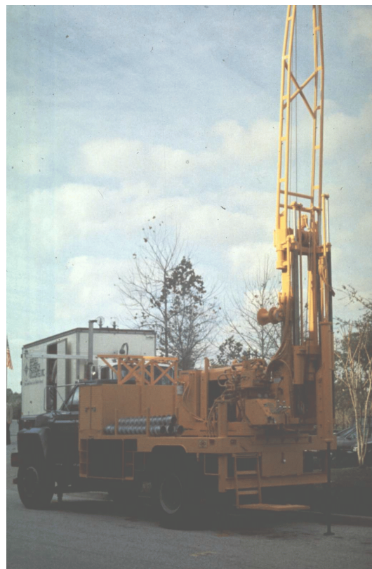
Figure 3-25. Views of Rotary Drill Rigs Mounted on Trucks for Soil & Rock Exploration.
