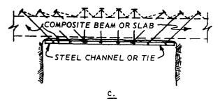
Figure 2-7. Beam or slab concept.
