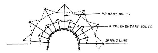
Figure 2-9. Supplementary rock reinforcement.
