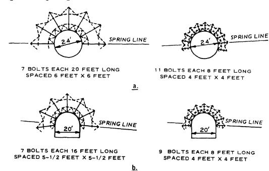
Figure 2.8. Arch concept of rock reinforcement.
