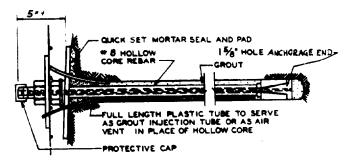
Figure B-2. Rock bolt deformeter.
