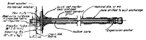
Figure B-1. Grouted rock bolt (with chain link fabric).
