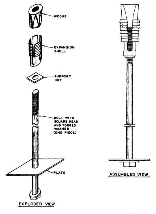
Figure 3-2. Regular expansion anchorage--headed bolt.
