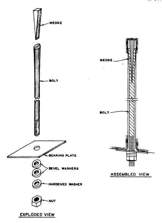
Figure 3-1. Slot and wedge rock bolt.
