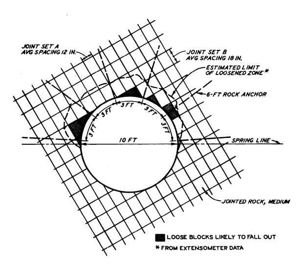
Figure 3-13. Example of underground reinforcement.
