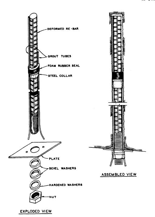
Figure 3-6. Grouted end anchorage, pumpable type.
