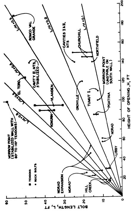
Figure 7-4. Bolt lengths used on cavern walls.
