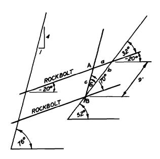
Figure 3-16. Calculation of actual bolt spacing for FS = 1.1.
