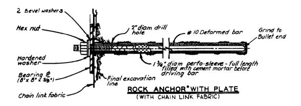
\* ON LONG ANCHORS, CENTER LUGS SHOULD BE WELDED TO THE BAR SO THAT THEY WILL CENTER THE BAR AND ALLOW GROUT TO FLOW COMPLETELY AROUND THE ANCHOR BAR.
