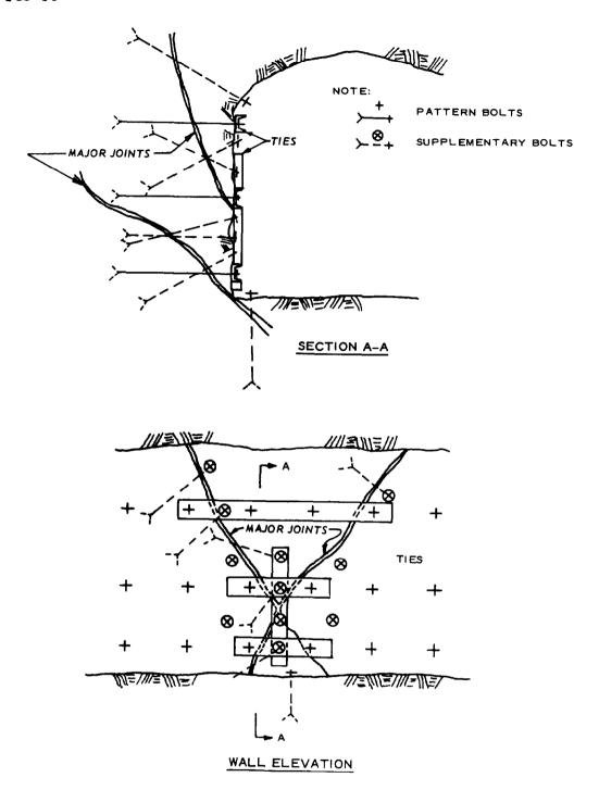
Figure 6-3. Typical use of ties and supplementary bolts.
