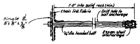
Figure B-3. Supplementary bolts for chain link fabric.
