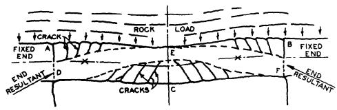
Figure 2-4. Mode of failure of uniform material beam.
