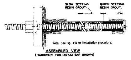
Figure 3-9. "Thread bar" rock bolt with polyester resin grouted anchorage.
