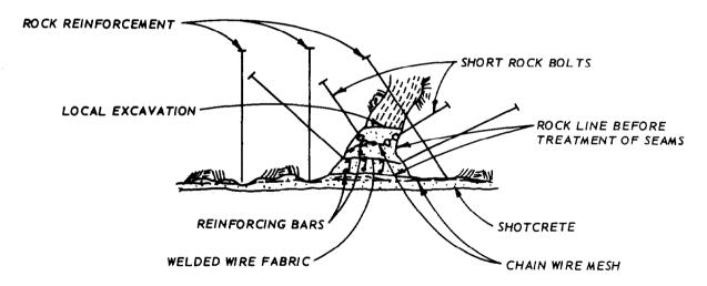
Figure 6-2. Typical local structural treatment of wide seams and fractured zones.
