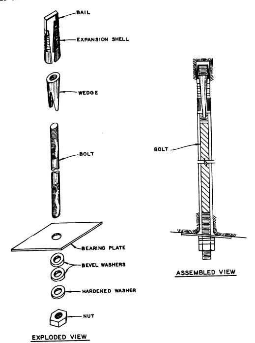
Figure 3-3. Bail expansion anchorage--solid bolt.
