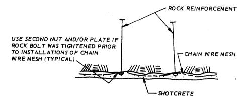
Figure 6-1. General surface treatment-wire mesh and shotcrete.
