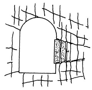
(b) Progressive partial failure of joint blocks adjacent to excavation surface.
