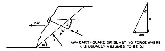
Figure 3-15. Force polygon for earthquake or blasting force.
