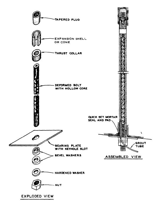
Figure 3-5. Hollow groutable deformed bar rock bolt.
