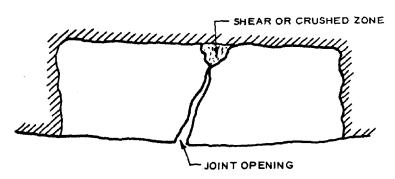
Figure 2-3. Failure by rotation.
