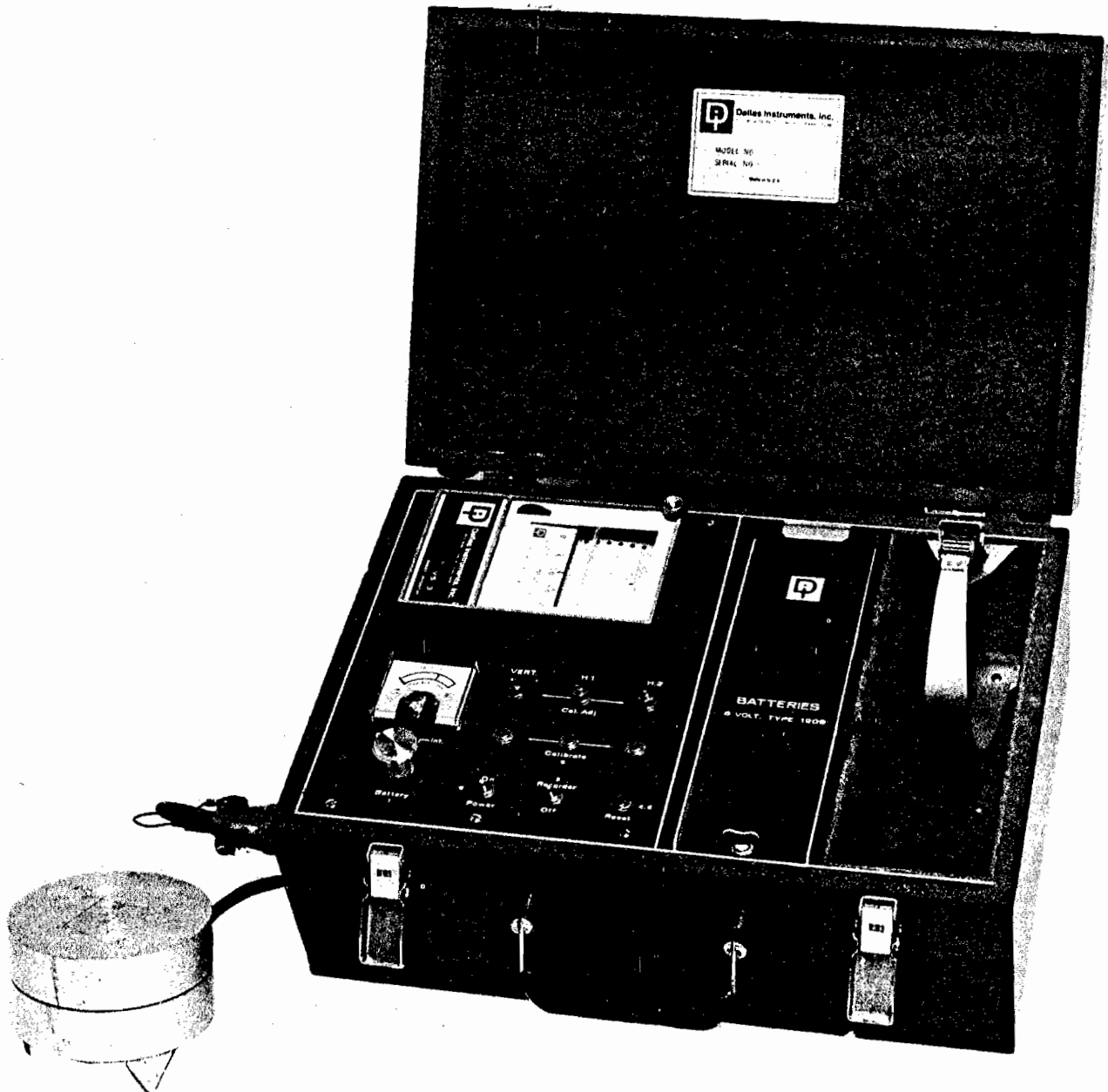
Figure 94.—Seismograph for measuring ground vibrations from blasting.
