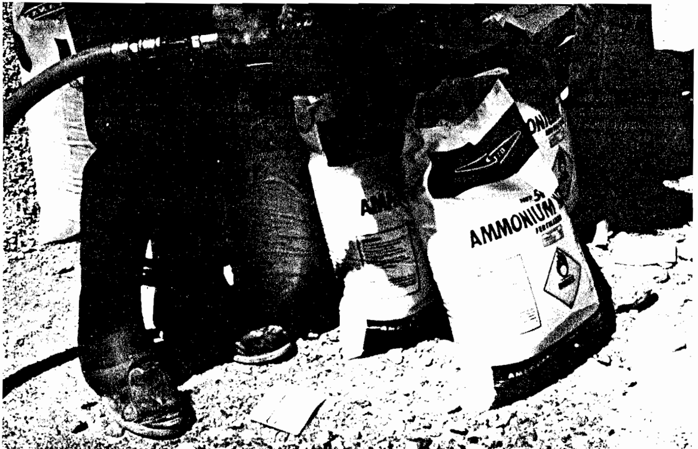
Figure 16.—Field mixing of AN-FO. (Courtesy Hercules Inc.)
