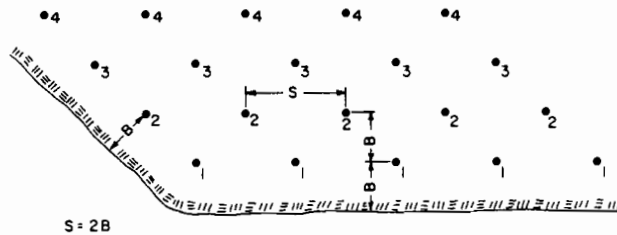
Figure 68.—Corner cut staggered blast pattern—Simultaneous initiation within rows (blasthole spacing, S, is twice the burden, B).
