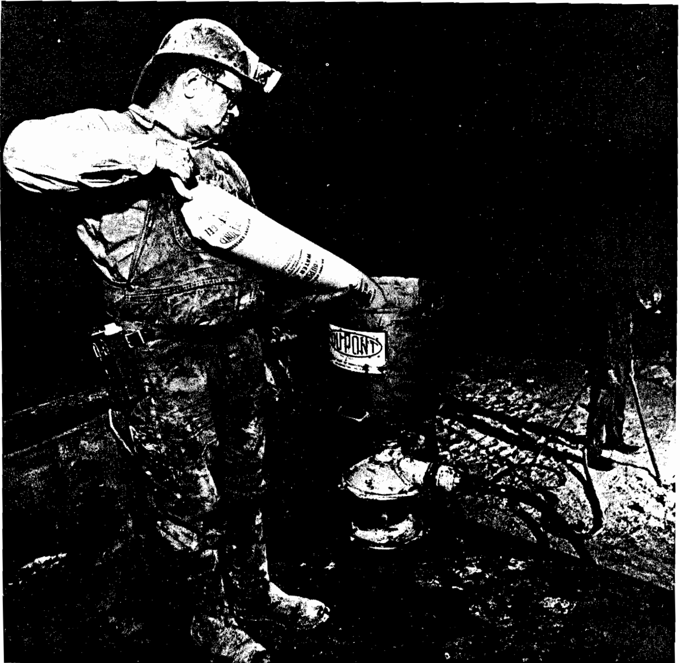
Figure 57.—Pumping slurry into small-diameter borehole. (Courtesy Du Pont Co.)
