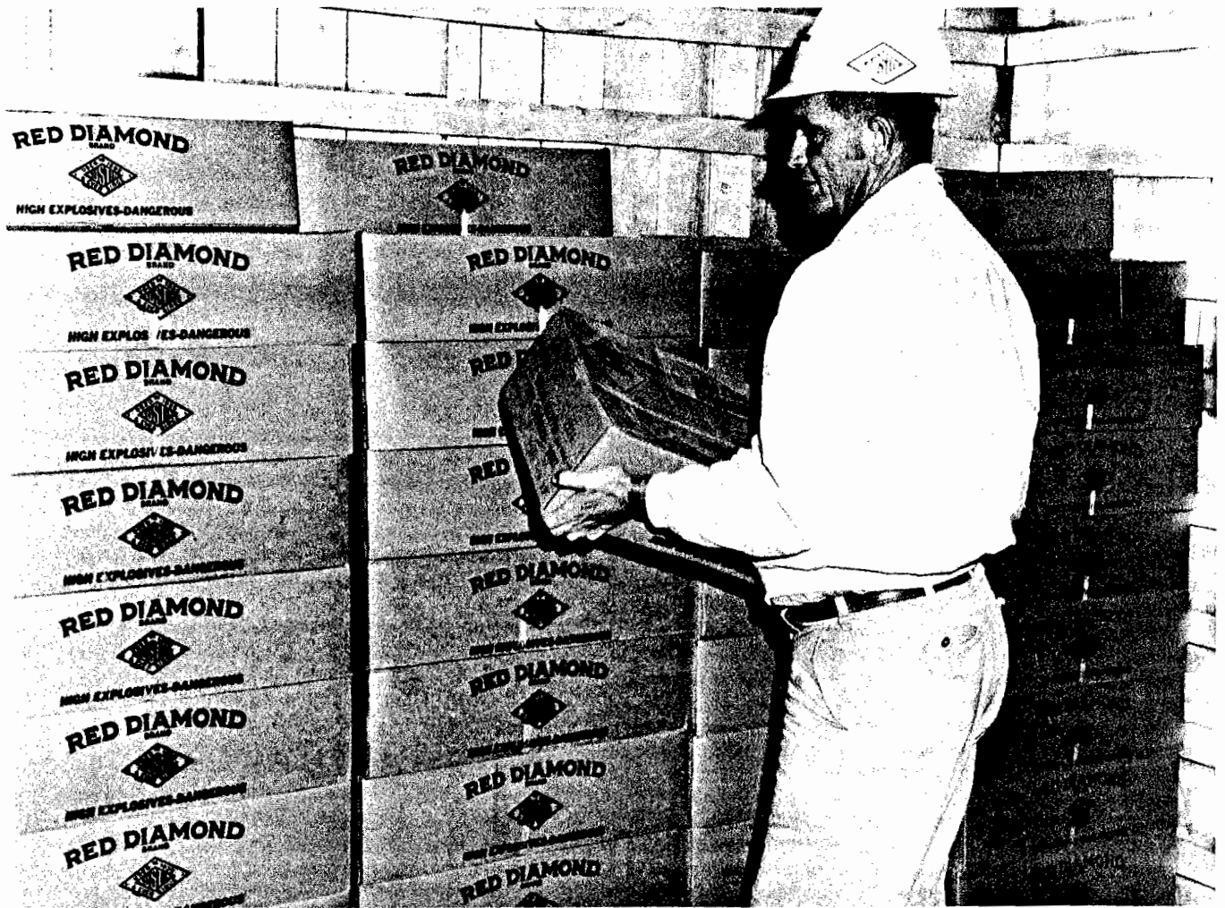
Figure 99.—Proper stacking of explosives. (Courtesy Austin Powder Co.)
