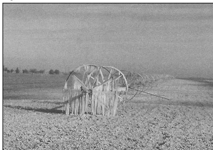
Figure 11-1. Side roll sprinklers apply potato processing wastewater throughout the winter at Aberdeen, Idaho. (Courtesy of Cascade Earth Science.)
