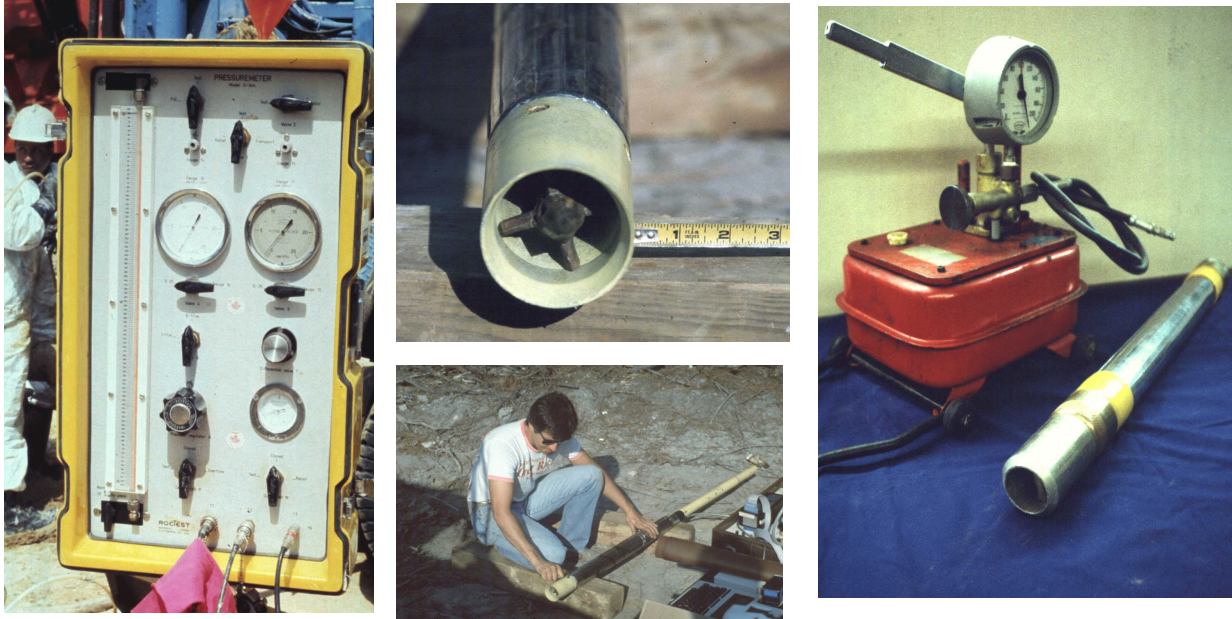
Figure 5-19. Photos of Pressuremeter Equipment, including Menard-type pressure panel, SBP probe, SBP cutter teeth, hydraulic jack, and monocell-type probe.
