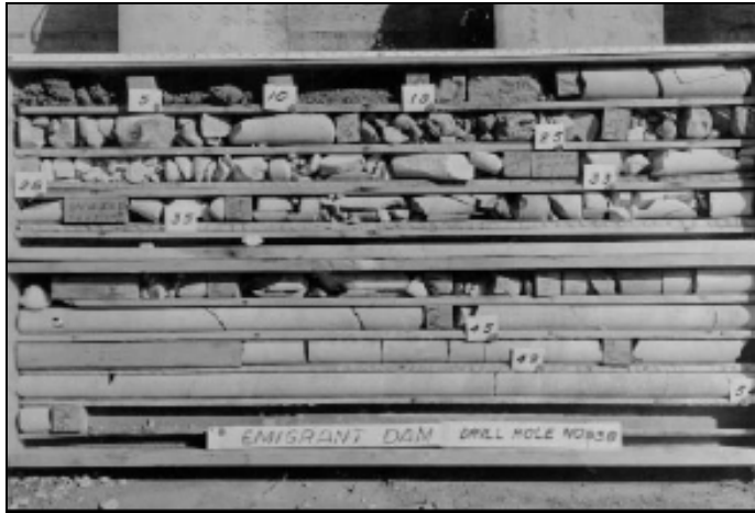
Figure 49. Arrangement of cores in a core box to ensure proper identification of samples.
