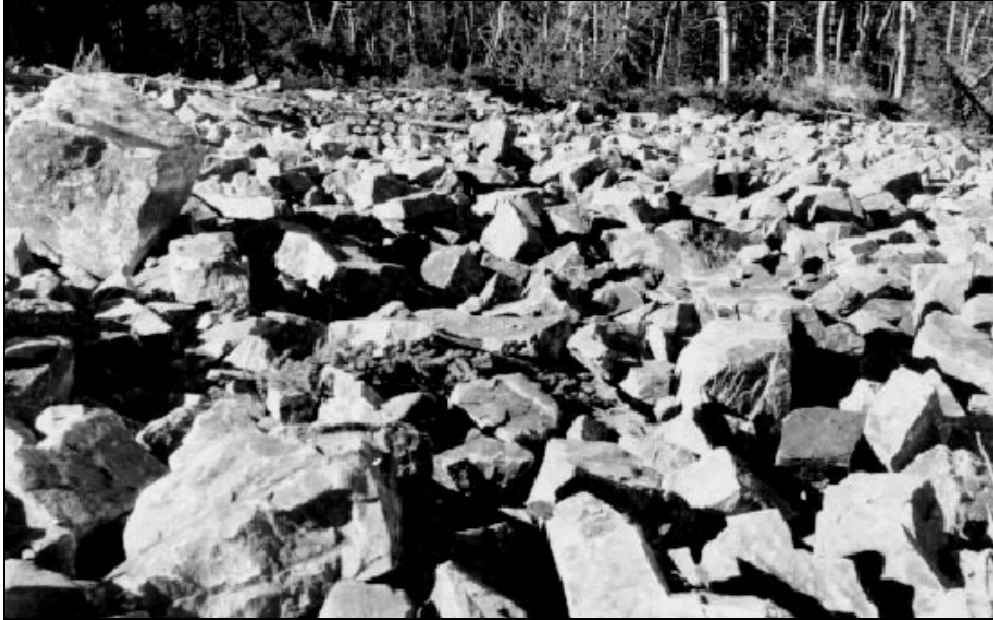
Figure 15. Results of a major blast in a riprap quarry.
