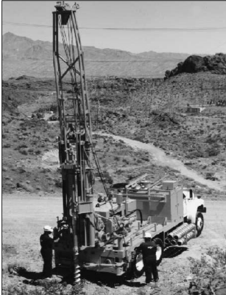
Figure 28. Photograph of typical rotary drill showing some of the essential equipment for rotary drilling.(Central Mine Equipment Company)
