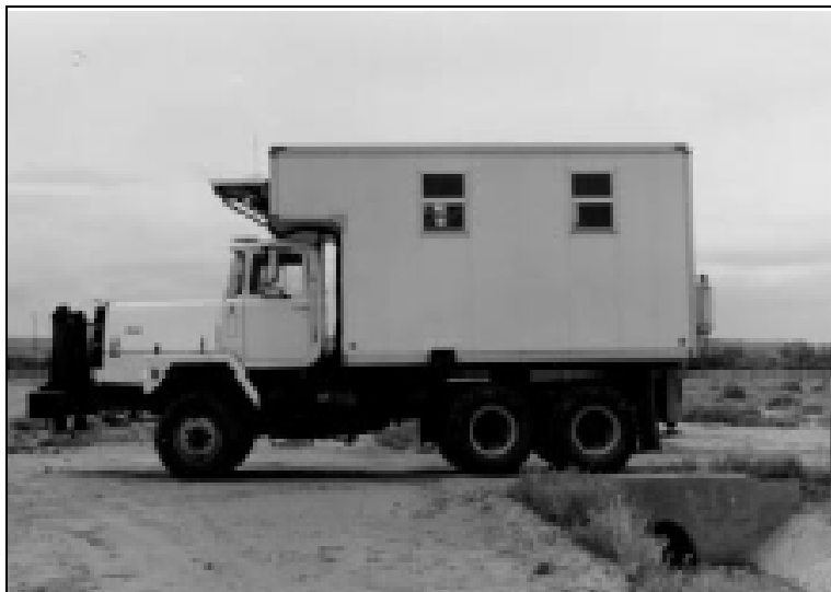
Figure 54. Electronic cone penetrometer testing vehicle.
