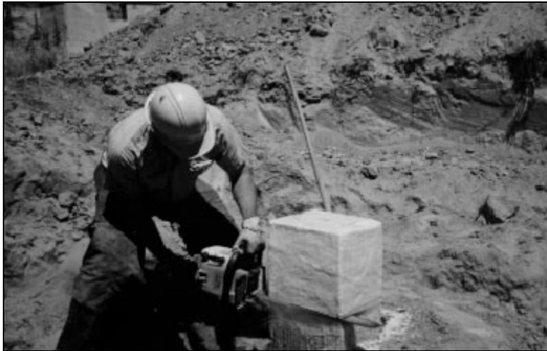
Figure 40. Chain saw equipped with carbide-tipped blade being used to cut block sample.
