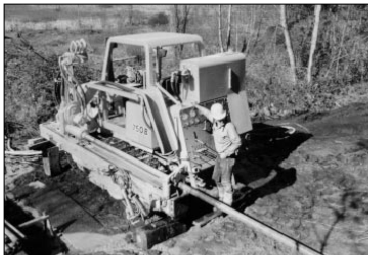
Figure 33. Horizontal rotary drill. Aardvark model 500 drill with adjustable box-beam slide, crawler-tractor mounted.
