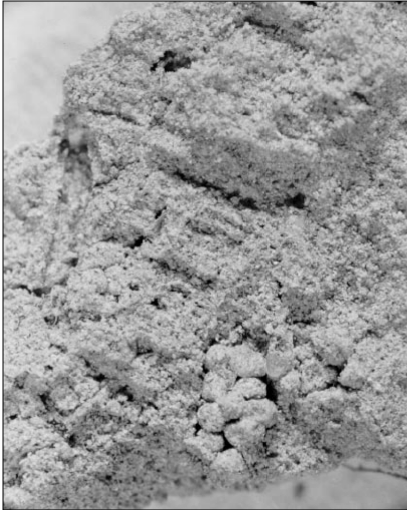
Figure 8. Photomicrograph showing typical open structure of silty loess.
