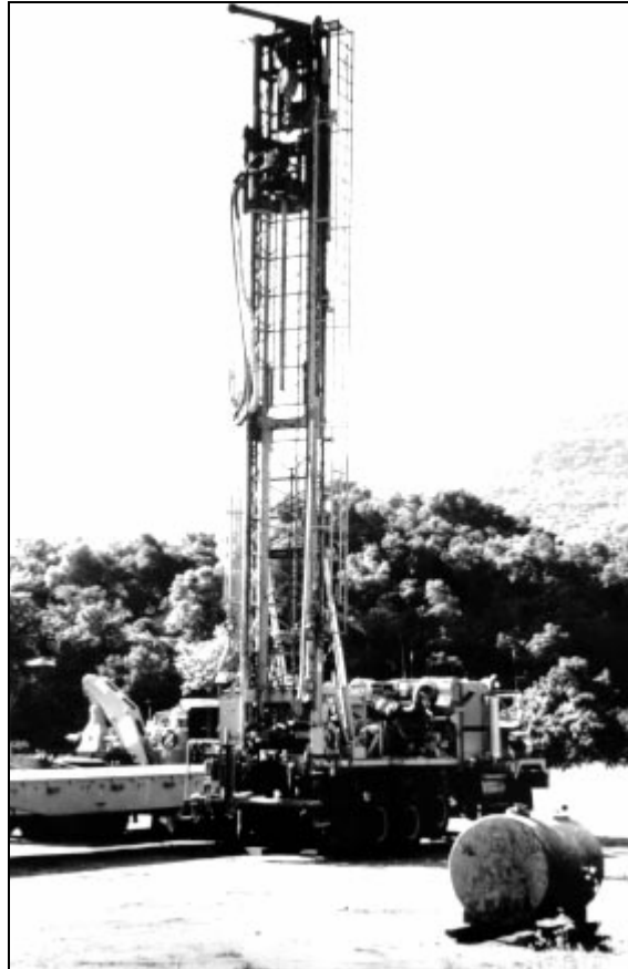
Figure 29. Top-head drive drill with head-in mast for drilling.
