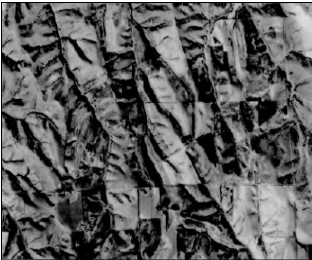
Figure 7. Aerial view and topography of loess identified by smooth silt ridges; usually parallel, right-angle drainage patterns; and steep-sided, flat-bottomed gullies and streams.
