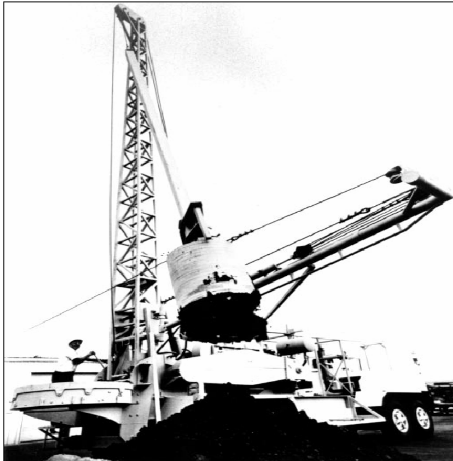
Figure 25. Bucket drill rig in drilling position with a 24-foot triple Kelly and 36-inch bucket.
