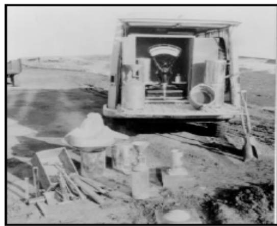
b. Type V laboratory—vehicle equipped for on-site earthwork control tests.
