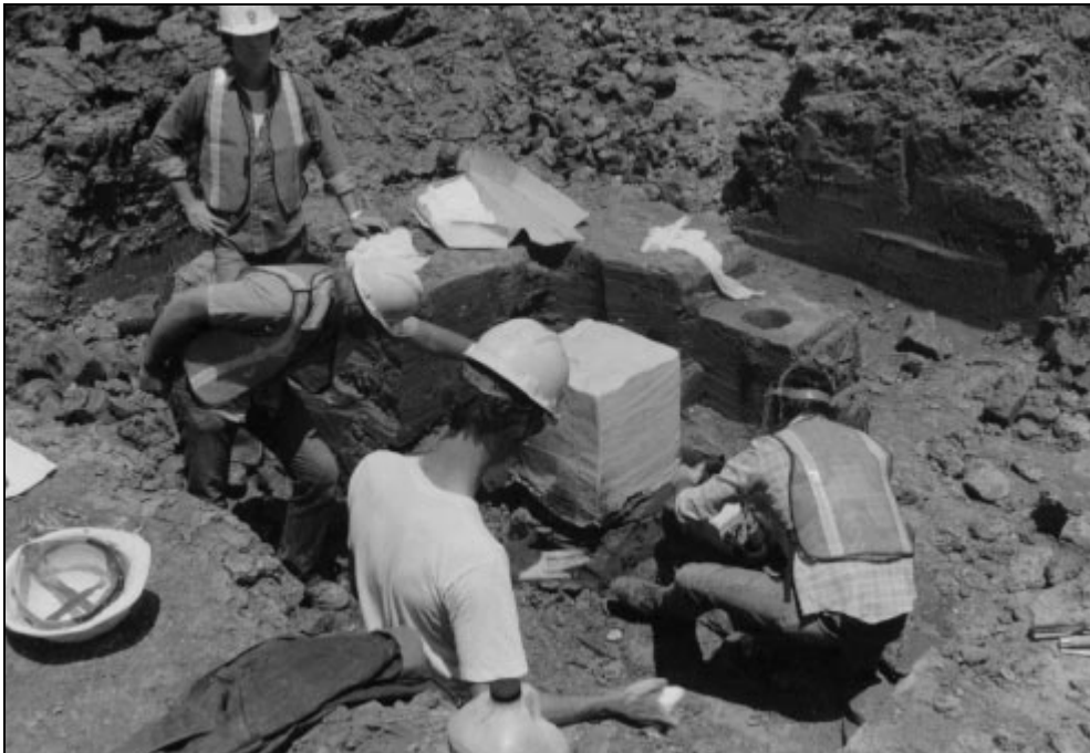
Figure 26, Block sample from test pit in zone 1. Final saw cut being made beneath the sample with a chain saw equipped with special tungster carbide bit.
