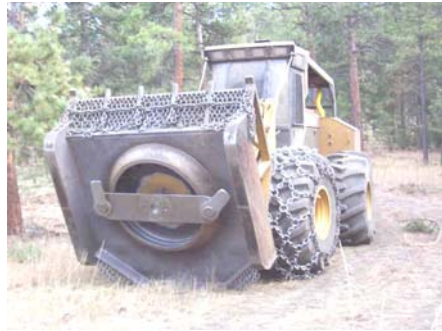
Figure 7: Hydro-Ax Mower Cutting Deck Bottom
