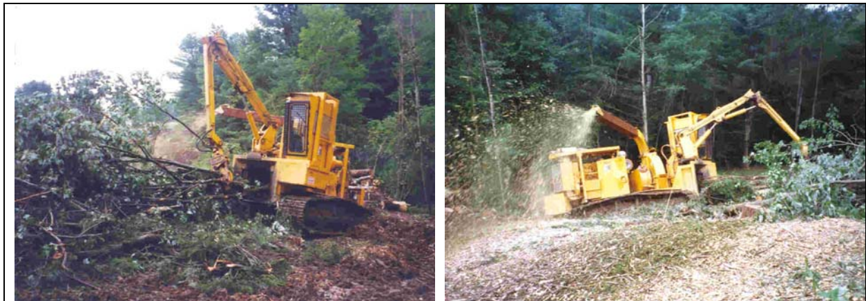
Figure 10: Mechanical Feed Chipper (two views)
