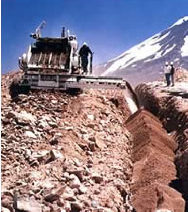
Figure 29: “Ozzie” Type Padding Machine Self Feeds from the Spoil Pile
