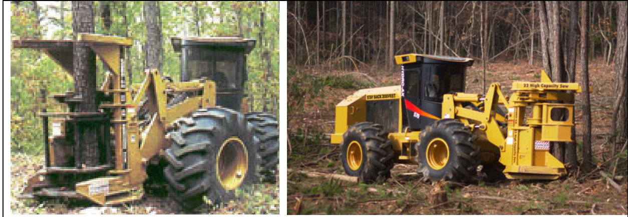
Figure 9: Hydro-Ax Tree Cutter (two views)
