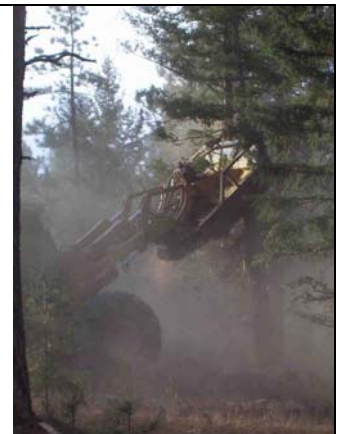
Figure 8: Hydro-Ax with Active Elevated Cutting Deck
