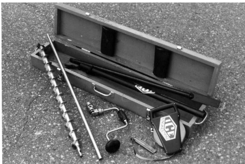
Figure 16-8. Standard CRREL ice thickness measuring kit.
