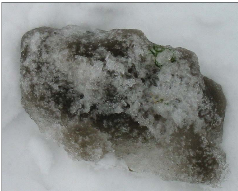
Figure 7-6. Sediment-laden frazil slush taken from Flat Creek in Jackson, Wyoming (photo by S.F. Daly, CRREL).
