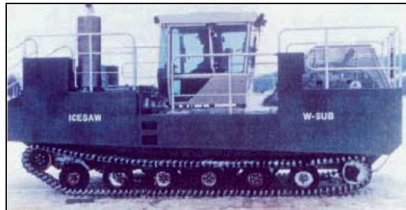
Figure 3-3. ICESAW used for cutting river ice (photo courtesy of Mobimar, Ltd.).
