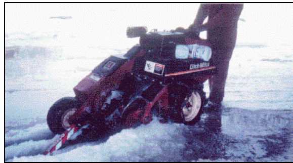
b. Ditchwitch 1260 cutting ice in Montpelier, Vermont.
