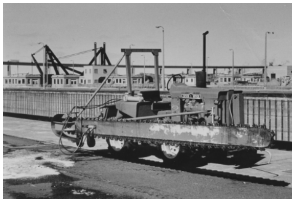
Figure 18-19. Ice cutting saw at Poe Lock.
