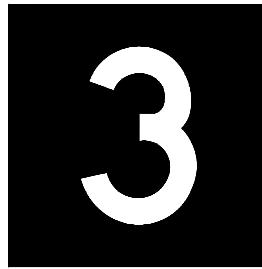
Figure 15. Runway Distance Remaining Sign
