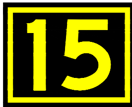
b. Runway Location Sign
