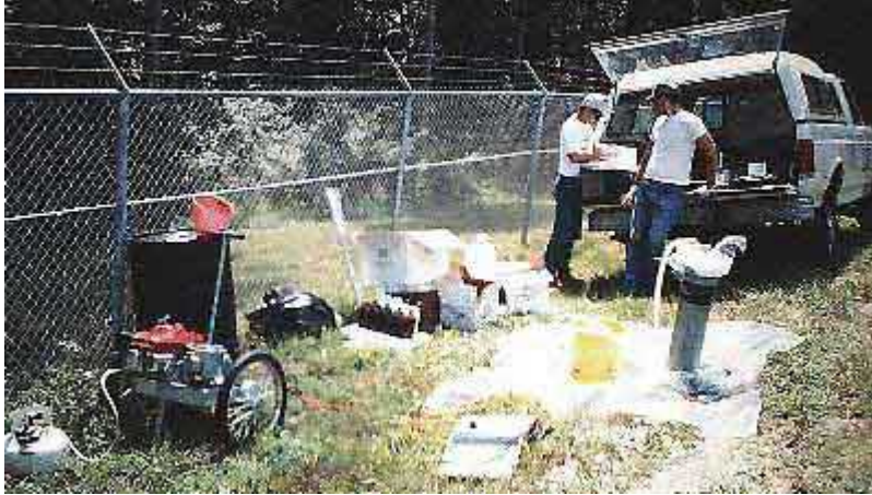
Figure 7: A well being prepared for groundwater sampling at the waste disposal site.
