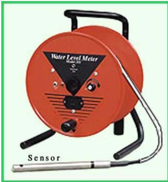
Figure 6: Electronic Water Sensing Device to Measure Groundwater Level in Wells
