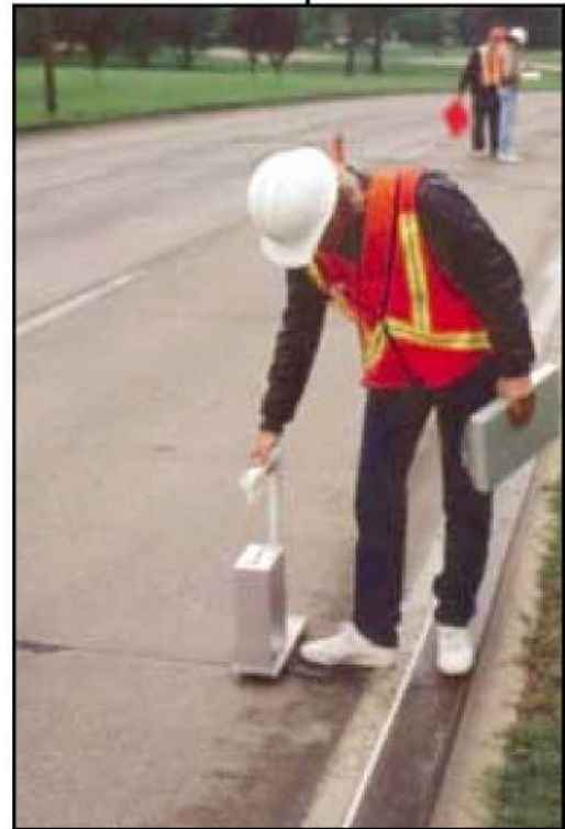
FIGURE B1 The Georgia Faultmeter in Use
