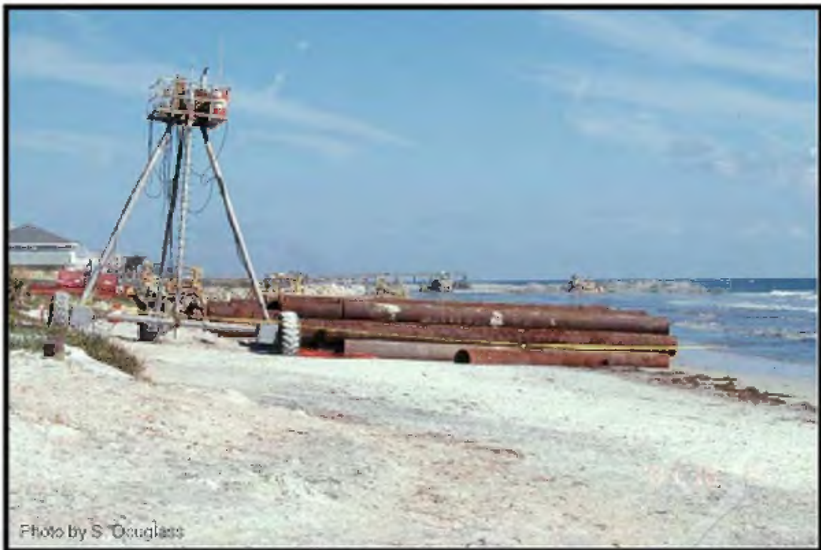
Figure 5.11. A CRAB (Coastal Research Amphibious Buggy) used to measure beach profiles during beach nourishment
