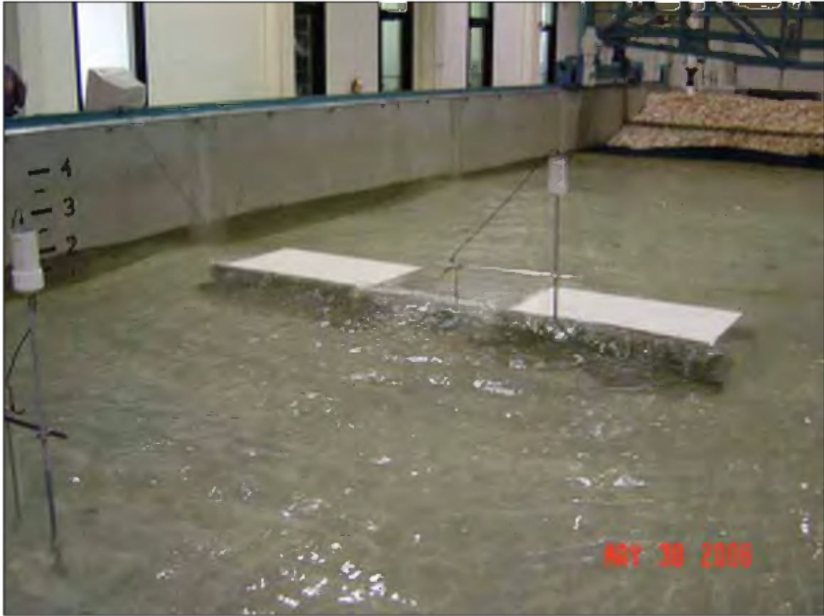
Figure 5.23. Physical model test of wave loads on bridge decks (Texas A&M photo)
