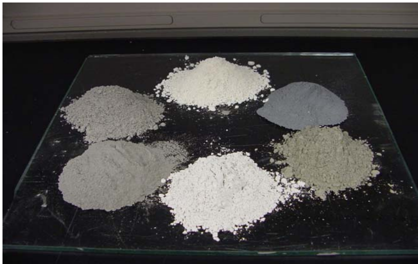
Photo 6.3.2-1 Cement and supplementary cementitious materials
