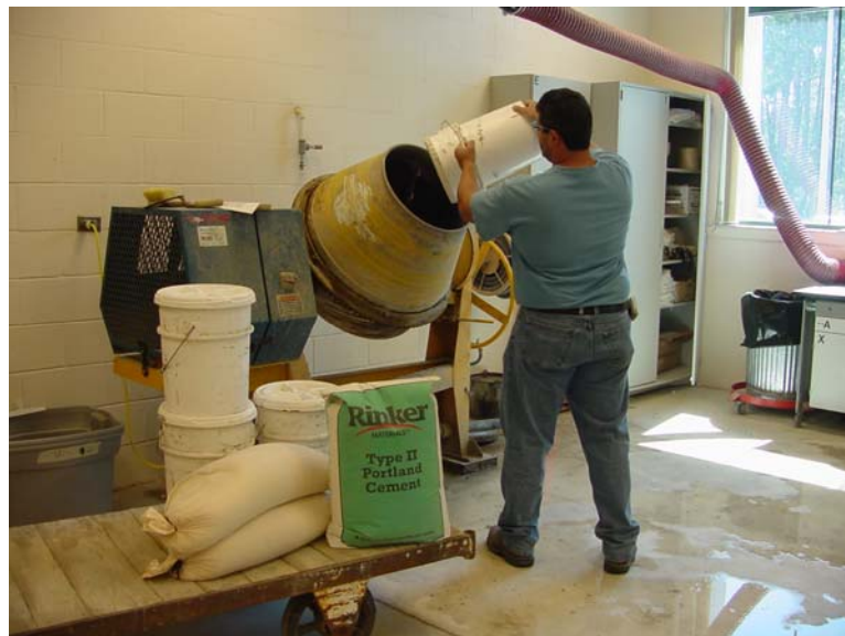
Photo 6.3.2 -2. Trial batching concrete mixtures.
