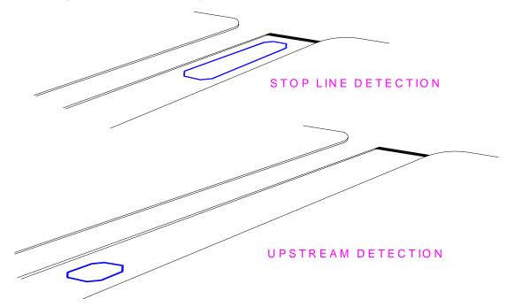
Upstream detection is typically used on higher speed approaches to provide dilemma zone protection (to be discussed later) while stop line detection is typically used on lower speed approaches and in left turn lanes. It is common to find short, upstream detection areas on the high speed approaches to an intersection and long, stop line detection areas on the lower speed approaches, and in the left turn lanes.
