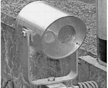
Whereas the detector unit for buried detection is typically located in the controller cabinet, the detector unit for overhead installations is often an integral part of the field unit. In these overhead installations the lead-in wire does not connect the field unit to the detector but rather connects the field unit/detector assembly to the controller or to some other pre-processor located in the controller cabinet.
