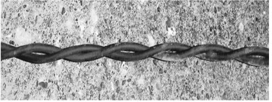
Shielded lead-in cable is typically constructed of number 14 or number 12 AWG (American Wire Gauge) wire that is twisted at approximately 15 twists per foot and is covered by an aluminum-polyester shield and encased in a continuous PVC (PolyVinyl Chloride) outer jacket.
