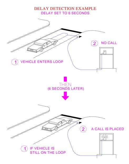
Detectors can also be purchased which allow the call to be extended even after the vehicle has left the detection area. The amount of this extension is also a user-
