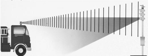
When the optical signal is received, the detector will cause the traffic signal controller to implement a special preemption plan that provides the green indication
