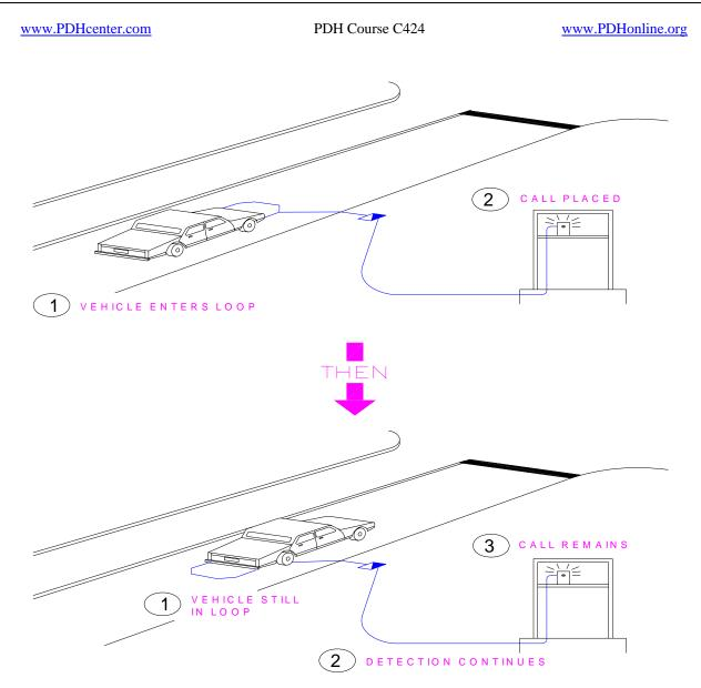
The call will not "drop" (cease) until the vehicle totally vacates the detection area. If the phase is currently green, then the green period will be extended by this call. If the phase is currently red, then the controller will continue to recognize the call as long as the vehicle is in the detection area. Presence detection is typically associated with long stop line detection areas programmed for non-locking operation.
