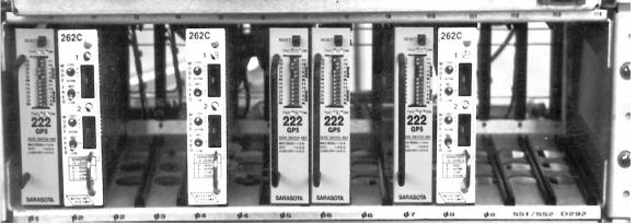
Detectors can also be purchased as either single-channel or multi-channel units. It is not unusual to find up to four channels on a multi-channel detector, with each channel monitoring a separate loop assembly.
