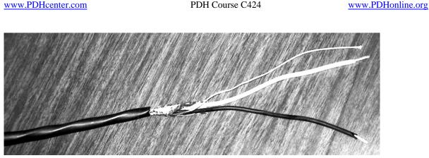
This construction allows loop wires for different detectors to run in the same conduit for long distances without causing interference problems.
