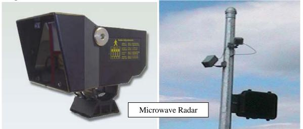
Passive devices detect the presence of a pedestrian without requiring the pedestrian to push a button.
