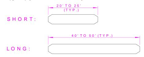
Short detection areas are typically less expensive and easier to construct than long detection areas. In addition, they are quite suitable for certain types of detection designs, such as those used on high speed approaches. Long detection areas have
