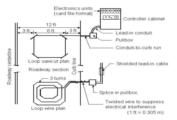
Between the loop and the lead-in cable, the unshielded loop wire should be twisted at no less than 5 twists per foot. Twisting the wires cancels their inductance field, ensuring that inappropriate vehicle detections do not occur.
