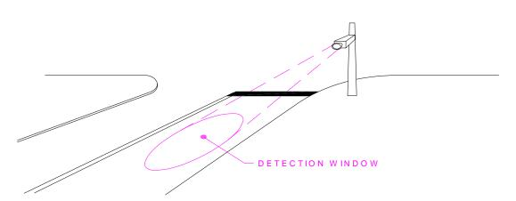
In order to have a stable detection area, the unit must be mounted overhead on a pole; it cannot be allowed to swing free on a span wire if reliable detection is to be provided. Overhead detection units are typically mounted directly over the travel lane on a mast arm, or are mounted off to the side of the lane on a pole. However, at wide intersections, providing accurate detection for main street left turn lanes can be difficult unless long mast arms are present or a median pole exists.
