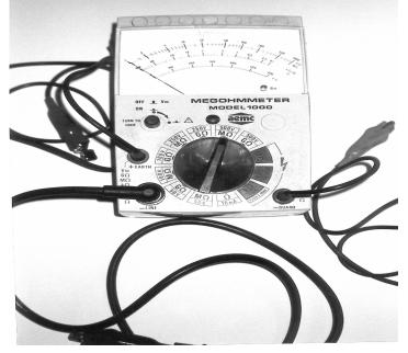
The continuity of the inductance loop assembly is tested by connecting each end of the loop to the meter and reading the resistance of the assembly in ohms. A low resistance (less than 2 ohms) is desired, which is indicative of a continuous loop assembly with no breaks in the wire. A resistance value of greater than 5 ohms is typically considered unacceptable.
