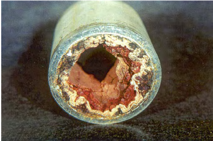
FIGURE 3-5. Scaled Boiler Tube
