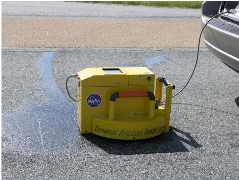
Figure 2-20 Photo of Dynamic Friction Tester (courtesy of Nippou Sango Co, Ltd) ( www.nippou.com )
