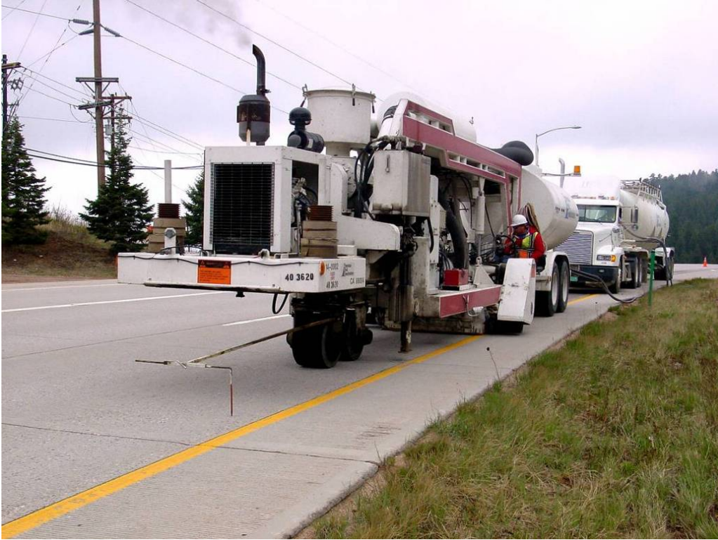
Figure 5-8 Typical grinding machine, front view (Courtesy of Caltrans)
