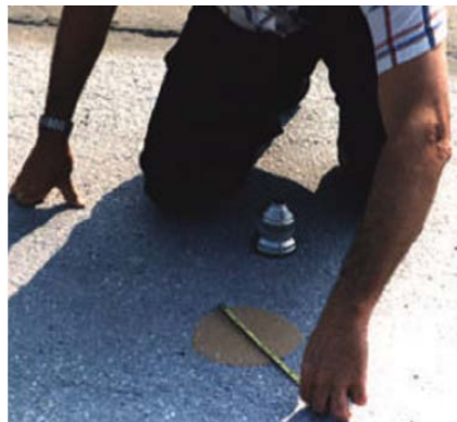
Figure 2-9 Photo of original “sand patch” test using Ottawa sand and spreading tool (Hoerner and Smith, 2002)
