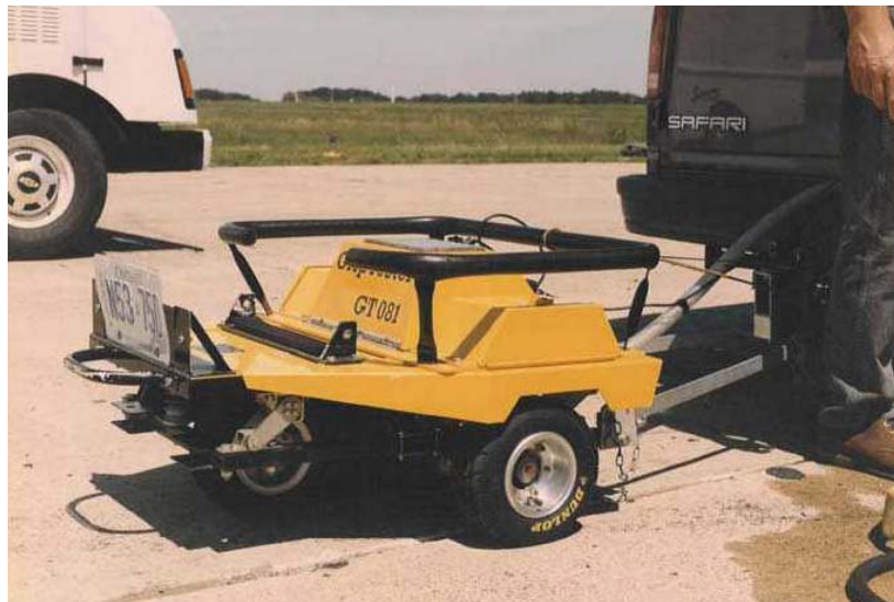
Figure 2-16 Photo of GRIPTESTER-towed mode (Wambold and Henry, 2002)
