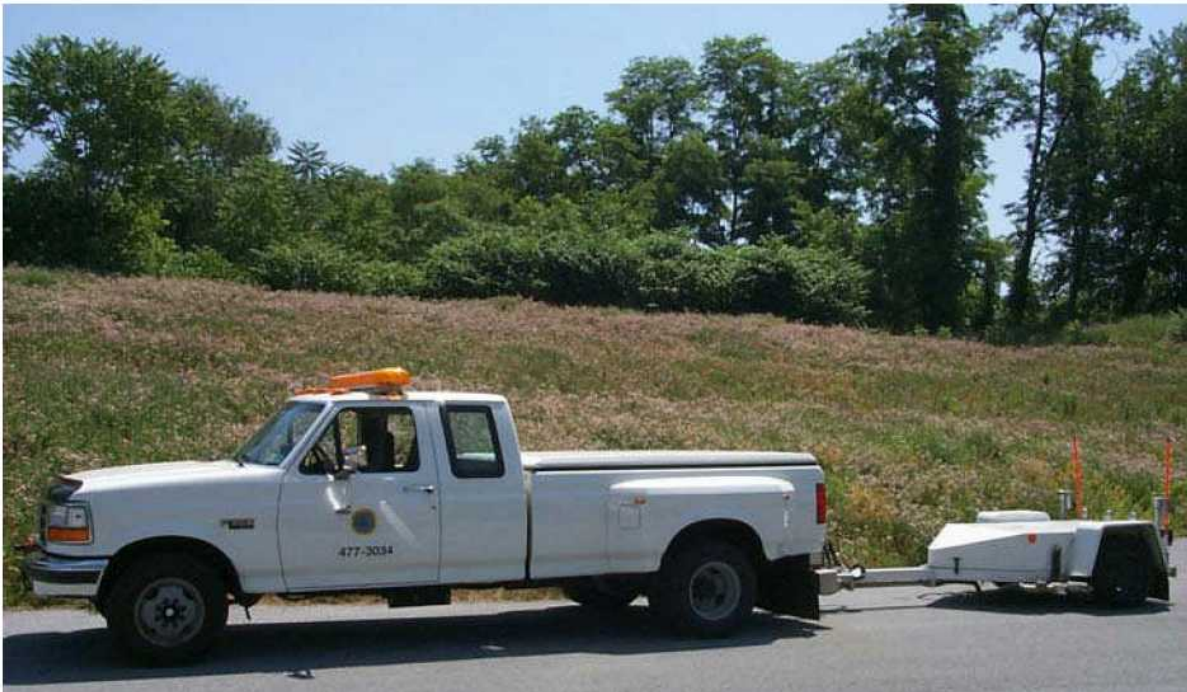
Figure 2-13 Pennsylvania DOT E-274 locked-wheel friction tester (Wambold and Henry, 2002)
