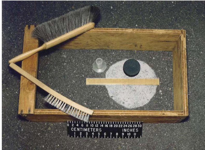
Figure 2-10 Photo of volumetric texture depth (“sand patch”) test equipment with glass beads and a hockey puck (Wambold and Henry, 2002)
