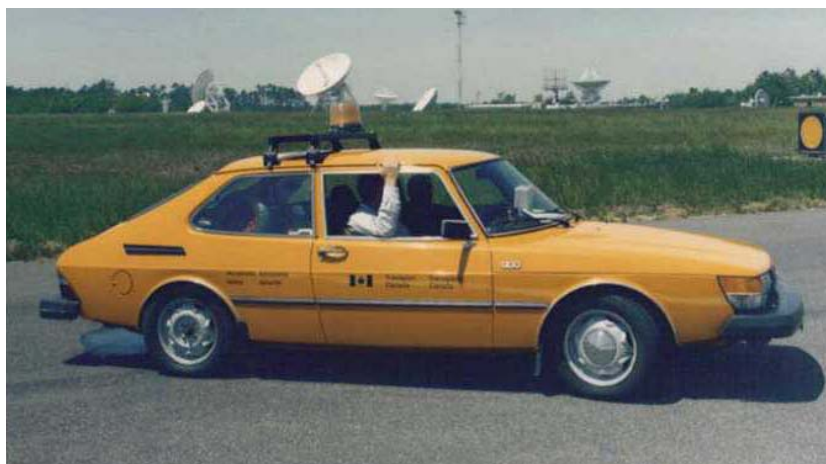
Figure 2-17 Photo of SAAB Surface Friction Tester (Wambold and Henry, 2002)
