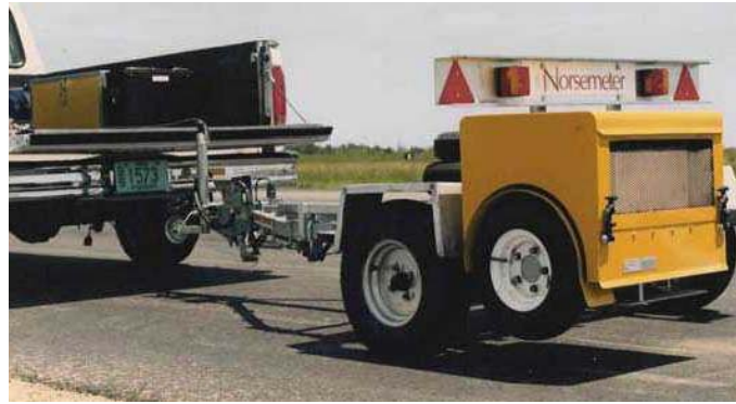
Figure 2-18 Photo of Norsemeter ROAR – Variable Friction Tester (Wambold and Henry, 2002)
