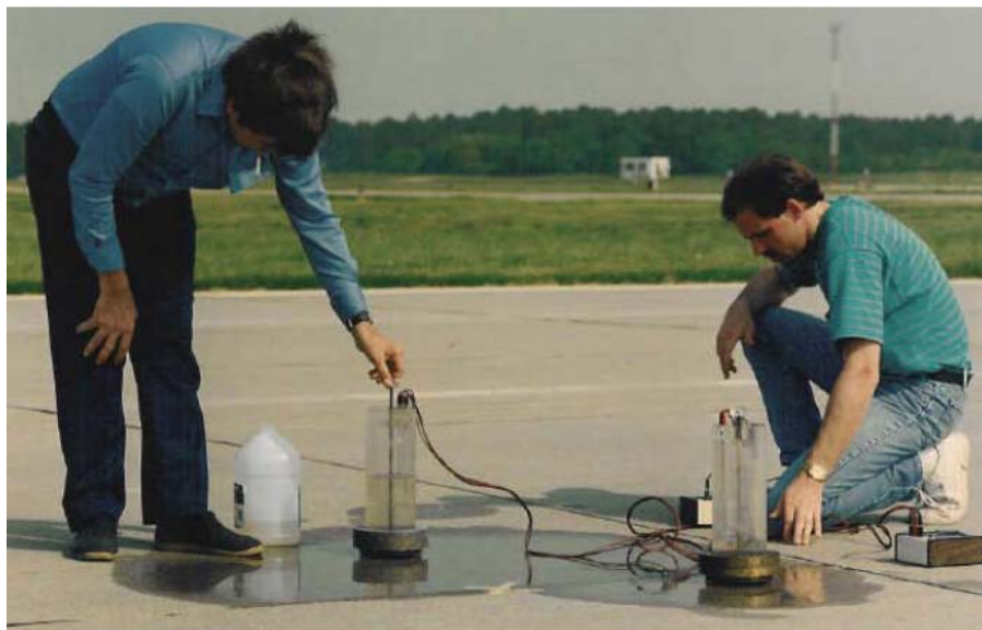
Figure 2-12 Photo of Outflow Meter in use (Wambold and Henry, 2002)
