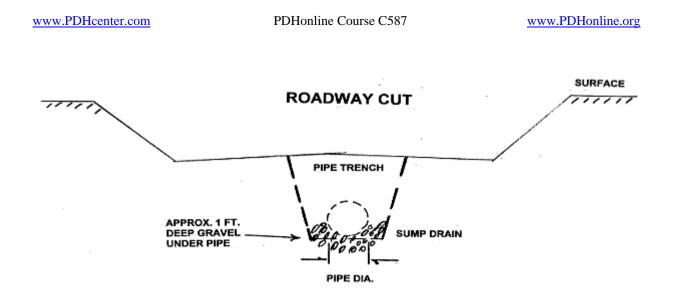
A sump pump of appropriate size can be used at the low point of the pipe installation, most likely with a shallow "well" which is cut two or three ft. below the pipe bottom and filled with gravel. Should ground water flow prove to be substantial, more than one such "well" may be required, along with additional pumps or pumping capacity.
