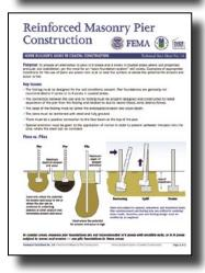
Fact Sheet No. 14, Reinforced Masonry Pier Construction – Provides an alternative to piles in V zones and A zones in coastal areas where soil properties preclude pile installation, but the need for an "open foundation system" still exists. Includes recommendations for good masonry practice in coastal environments.
