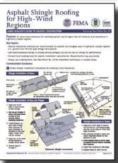
Fact Sheet No. 20, Asphalt Shingle Roofing for High-Wind Regions – Recommends practices for installing asphalt roof shingles that will enhance the wind resistance of roof coverings in high-wind, coastal regions. Issues include installation at hips, eaves, and ridges; shingle characteristics; weathering and durability; and wind resistance.
