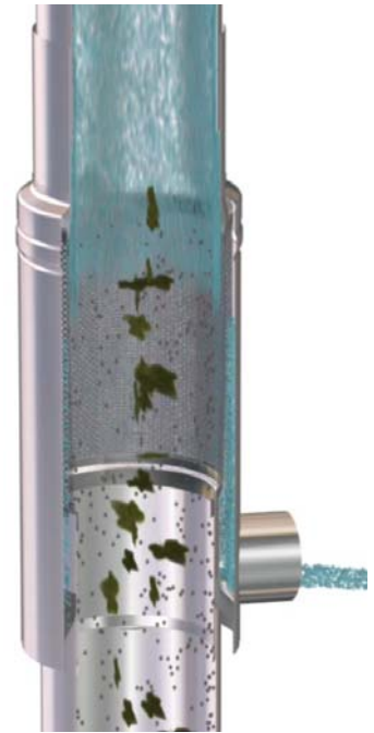
Figure 10: Vertical Inlet Device
