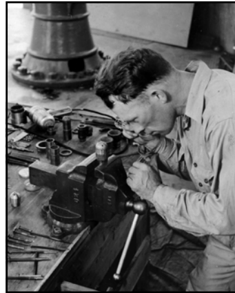
Drill bits were inspected with a magnifying glass before and after use (to check on alignment and/or fractures)
