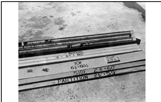
Cores (from A-4 and other holes) were preserved in boxes similar to the one above (they were made out of plywood; June 1939)
