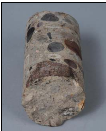
Concrete cores were taken in 1995 for testing finding: "Hoover Dam's concrete has continued to slowly gain strength...a durable concrete having a compressive strength exceeding the range typically found in normal mass concrete." Because non-reactive aggregate was used, the concrete of Hoover Dam is not subject to Alkali-Silica Reaction (ASR) which can/does cause deterioration in concrete structures such as occurred at downstream Parker Dam .
