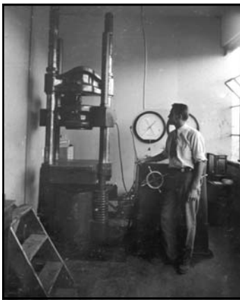
Southwark testing machine (for making tension and compression tests on weld specimens), Babcock and Wilcox Company plant. Capacity of machine is 3K-pounds per square inch (October 1933)
