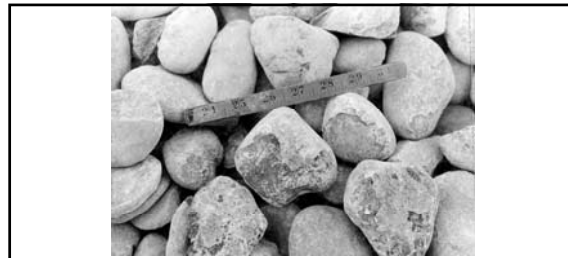
Course aggregate passed through Six Companies' gravel screening and washing plant in test run (February 12 th 1932). Concrete consists of four ingredients; sand and stone aggregate, water and Portland Cement. These must be mixed in the proper proportions to yield strong concrete. Aggregate is perhaps the most important of the materials in the concrete because it made up as much as three-quarters (75%) of Hoover Dam's mass. As well, the aggregate must be clean and free of clays, salts and organic matter. 574
