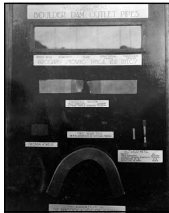
Display board showing pipe weld specimens (prepared by the Babcock and Wilcox Company; November 1934)
