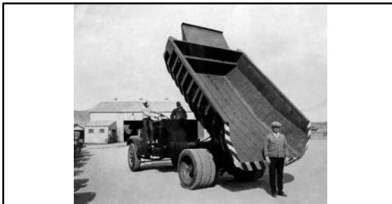
Mack truck; fourteen cubic yards capacity (February 1932). This was the largest truck ever built on two axles and weighed 65K-pounds when fully loaded. Mack's popular "AC" models evolved through the 1920s and, in response to a demand for trucks with larger capacities and higher speeds, Mack introduced the "B" series in 1927. Pneumatic truck tires were introduced by both Goodyear and Dunlop in 1919. 249
