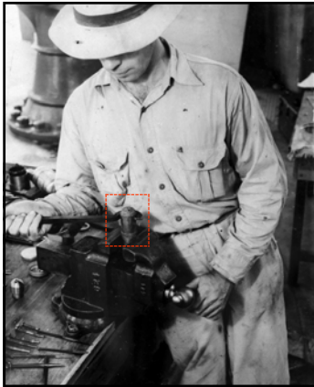
View showing a completed bit being removed from its temporary support (vise)
