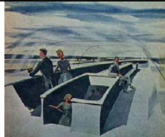
"Drawing of an observation platform in a plastic dome at the top of the arch. Visitors will be able to reach this lookout by train, elevator or stairs going up through the triangular legs of the arch. There will be two cable-operated trains. Each train, consisting of eight passenger capsules resembling automobile interiors, will move on a track up one leg of the arch and return by the same route."
