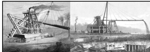
Left: caption: “‘Hercules’ Dredger for the Panama Canal.” A big job needed big machines. This big machine is a floating dredge. It digs up mud from the bottom of the river and dumps it on the side. The dredges traveled along the shallow rivers and made them deep enough for large ships to navigate.
