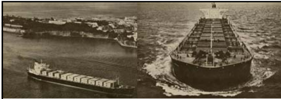
Left: caption: "A containership of the SEALAND fleet used for the carriage of containers exclusively" Right: caption: "The S.S. Cedros, one of the world's largest bulk carriers with a capacity of 170,418 DWT"
