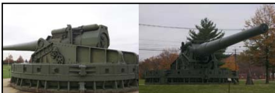
Above: 16"/ 50 (40.6 cm) Mark 3 Coastal Defense Gun on U.S. Army "Barbette" mounting; displayed at the Aberdeen Proving Grounds Museum in Maryland. The plaque reads;
