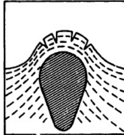
(d) A mound grows and then begins to dissociate, allowing vapor to filter through the broken material.
