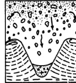
(f) The mound completely dissociates into fallback and ejecta, which are deposited to form the apparent crater and its lip.
