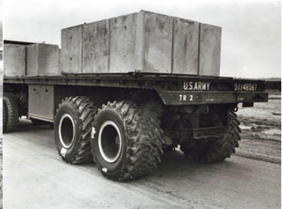
Top Left: caption: “AASHO Road Test - Illinois Off-Road Train Trailer used in the special test conducted after completion of regular test traffic.”
