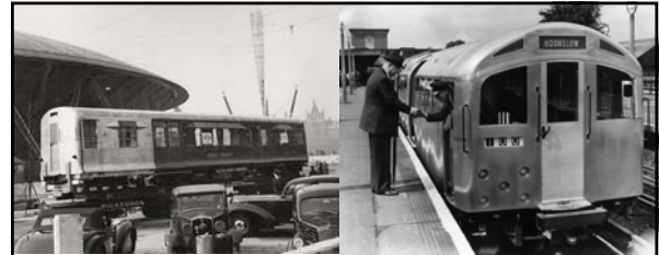
Top Left: when the District Line needed additional trains after WWII steel was in short supply so designers turned to aluminum. The resultant trains were called "R49 Stock." In the photograph (ca. 1951), a partially painted prototype arrives at the Festival of Britain site on the South Bank (the Dome of Discovery and Skylon can be seen in the background). The unpainted trains were put into service in 1953. Top Right: Sir John Elliott, Chairman of LTE, shakes hands with the driver of the new prototype "silver" tube train at Northfields station on the Piccadilly Line (August 1957) 258
