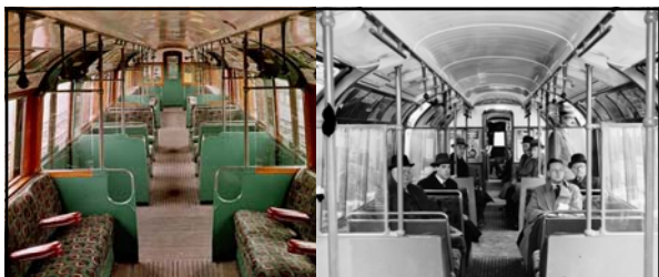
Top Left: the comfortable interior of a 1938 Stock car. These cars, which entered service in 1937/8, were a great improvement over their predecessors, boasting deep-cushioned seats covered in Woollen Moquette , slatted hardwood floors and art deco-style lampshades. They were hardwearing and still in good condition when this photograph was taken in the 1960s.
