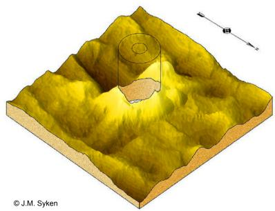
Ocean Surveys Inc. conducted an ultra high resolution multi-beam hydrographic survey of the lakebed adjacent to thirty Mackinac Bridge piers to generate an extremely detailed *Digital Terrain Model* (DTM) for the purpose of identifying and detailing scour activity. Data deliverables included contoured plan, isometric and profile presentations.
