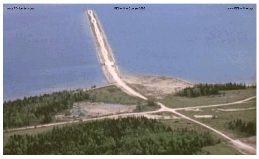
Above: a causeway 4,200-feet long was built from 1939 to 1941 in anticipation of a bridge across the Straits that was delayed due to the outbreak of WWII. Steinman used the existing causeway in his plans for the new bridge realizing a 135 savings of \$3 million in construction costs. 135 of 400
