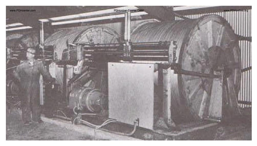
Above: caption: "Each reel weighed 16 tons and contained approximately 320,000 feet of wire. The wire was much stiffer than its appearance would indicate and was 0.192 inches in diameter – about as thick as a lead pencil." 285 © J.M. Syken
