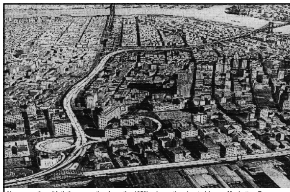
Above: caption: "Artist's conception from the 1950's shows the elevated Lower Manhattan Expressway looking east. In the foreground is the interchange with the Holland Tunnel, with the elevated West Side Highway running along the bottom of the photo. In the distance are connections with the William-341 sburg Bridge (top center) and the Manhattan Bridge (top right)."
