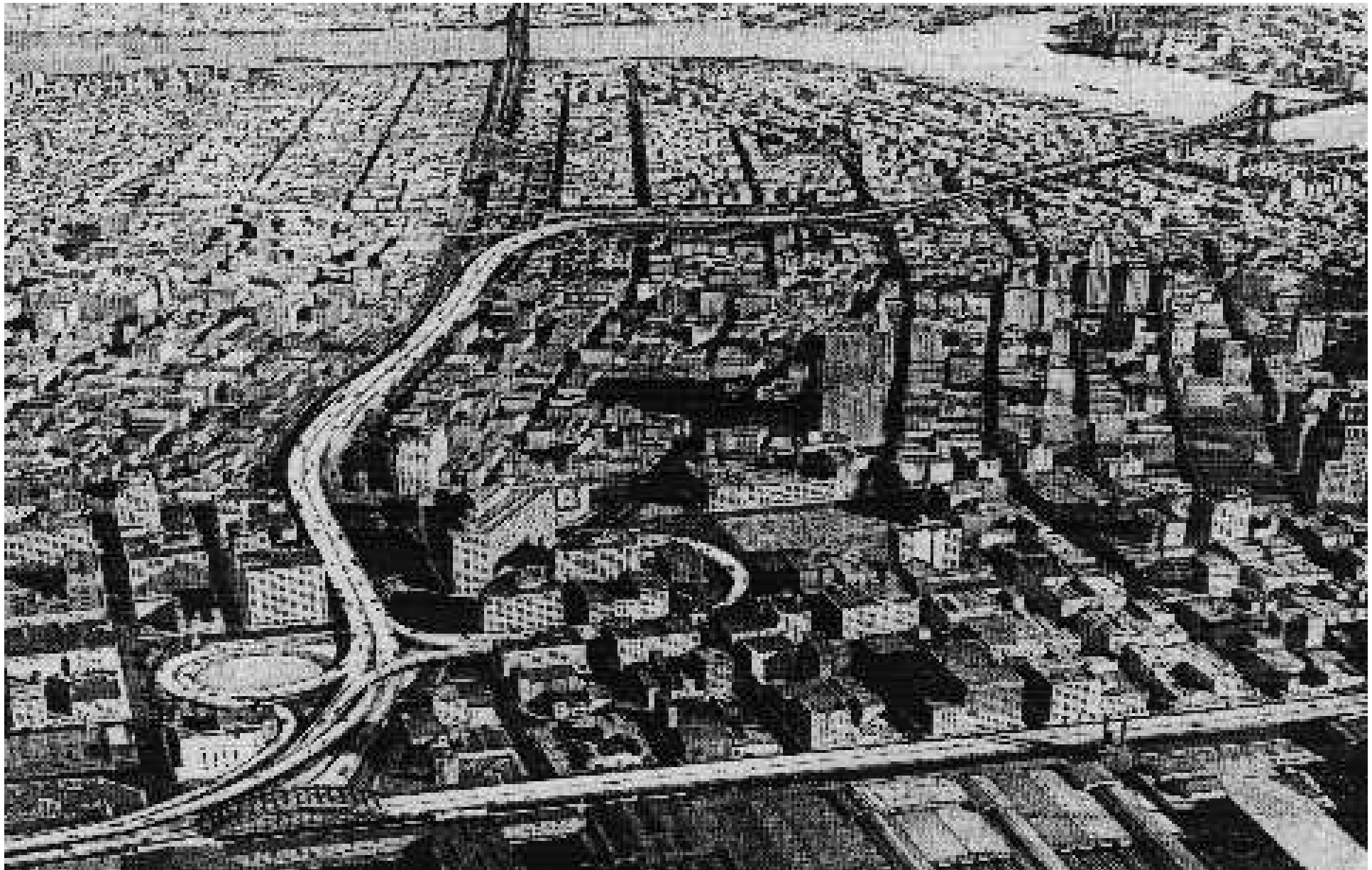
Above: caption: “Artist's conception from the 1950’s shows the elevated Lower Manhattan Expressway looking east. In the foreground is the interchange with the Holland Tunnel, with the elevated West Side Highway running along the bottom of the photo. In the distance are connections with the William- 723 sburg Bridge (top center) and the Manhattan Bridge (top right).”
