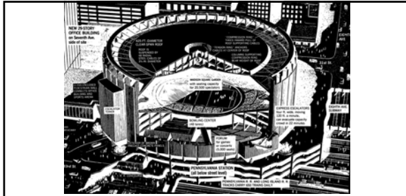
"A cable-suspended roof 425-feet in diameter, largest of its kind in the U.S., will dispense with supporting pillars and give spectators an unobstructed view from every seat of New York's new Madison Square Garden. Express elevators four feet wide will empty the arena of a capacity crowd in 22 minutes. Those are outstanding features of the $44 million sports center, shown in the cutaway view above, now rising on the Pennsylvania Station's 8½-acre site..." 295 Popular Science, May 1966
