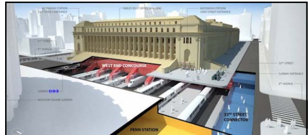
Above: caption: "MSDC rendering of the Moynihan Station and surrounding area." With the completion of Phase 1, passengers will be able to access Amtrak, New Jersey Transit (NJT) and LIRR trains through entrances at the Farley Post Office. This will alleviate passenger congestion in Penn Station and its surrounding streets. Specific work that is to be completed as part of Phase 1 includes:
