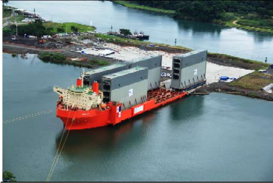
Deliver of lock gates to site laydown area
