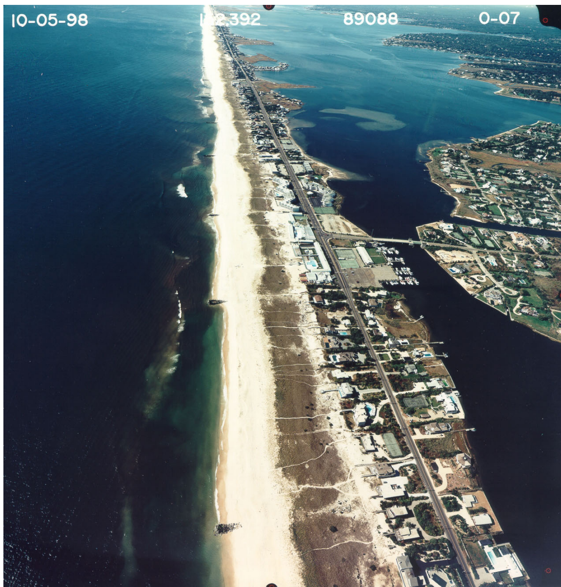
Figure V-3-30. Westhampton Beach, New York, groin field and renourished beach, 1998 (courtesy USAED, New York)
