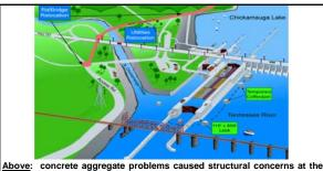
existing Chickamauga Dam Lock, resulting in the closure of the lock. As well, the existing 60-foot by 360-foot lock was a non-standard size that's not suited for the barges used by the modern transportation indus-try. The new 110-foot by 600-foot *Chickamauga Lock*, designed and constructed by the U.S. Army Corps of Engineers (Nashville District) will replace the existing lock, improve locking efficiency, and solve 470 the structural issues caused by the deficient concrete.
