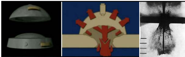
Above: caption: "A hollow, or shaped, charge is a concave metal hemisphere or cone backed by a high explosive, all in a steel or aluminum casing. When the high explosive is detonated, the metal liner is compressed and squeezed forward, forming a jet whose tip may travel as fast as 10 kilometers per second." In 1885, Charles Edward Munroe discovered what came to be known as the "Munroe Effect" (a/k/a "Neumann Effect") in explosives. He noted that a high explosive with a cavity facing a target left an indentation. The Munroe Effect was rediscovered by Ergon Neumann in 1911, but no practical applications were developed. Dr. Franz Rudolf Thomanek (working with Dr. Eric Schumann) developed the hollow charge weapon to take-out fortifications like Eben-Emael, where large cupped explosive charges placed atop armored cupolas would have devastating effect. 591
