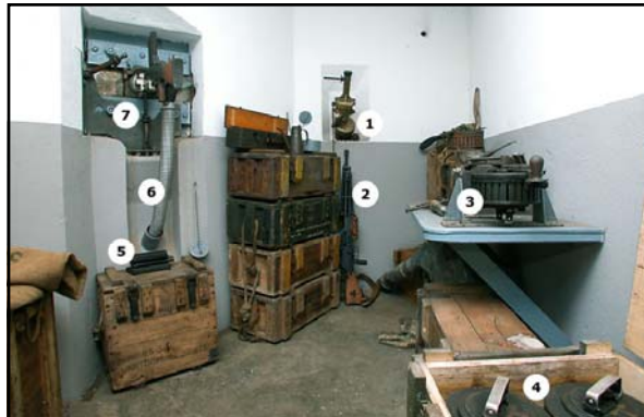
1) Grenade launcher (for defense of the ditch) 2) Automatic Rifle 3) Magazine loading device 4) Camemberts (magazines for the twin machine-guns) 5) Magazines for the Automatic Rifle 6) Flexible tube for spent cases 7) Type RB mounting 363
