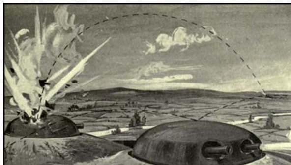
Above: caption: "Effect of Firing on Cupolas. Top dotted line shows the line of flight of siege howitzer shell, finally bursting on top of cupola, the range having been ascertained by the Germans long before war was declared. The bottom dotted line represents field-gun fire and shows shell glancing off cupola."
