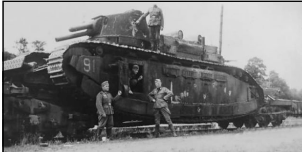
Above: caption: "The largest tank ever made: the French Char 2C (a/k/a "FCM 2C"), developed during WWI, used between 1921 and 1940. Only ten were built. This 69-ton tank was 33-ft 8-in long, 13-feet 5-inches high and 9-feet 10-inches wide and had a 75mm gun and four 8mm machine guns."
