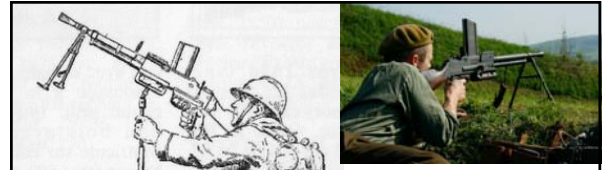
Above: caption: "A field army FM 24/29. Note the handgrip in front of the trigger which was absent on the Maginot models."
