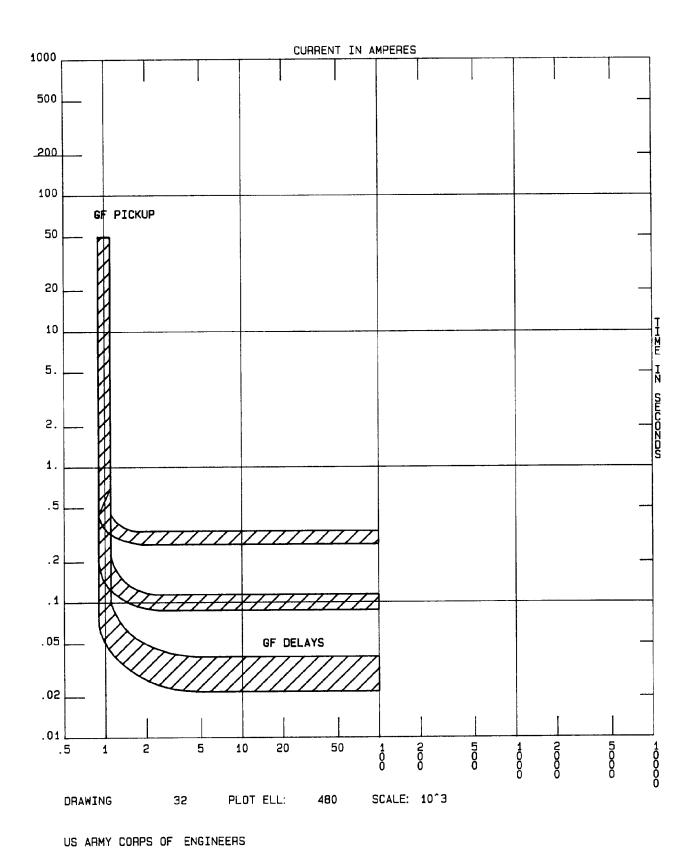
Figure 3-2. Solid state ground-fault characteristics.
