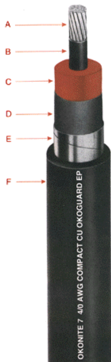
FIGURE 2 Copper Tape Shielded Cable Photo courtesy of The Okonite Co.
