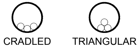
FIGURE 6 Cradled and Triangular Configurations
