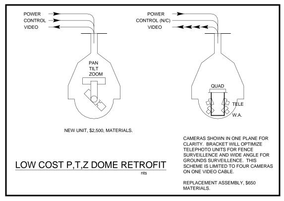
The many-camera large-dome above is based upon postage stamp cameras, available with telephoto varifocal lenses. Domes 9-in to 15-in can easily accept box cameras with longer telephoto lenses, as 7-70mm or 125mm. Four 3.6mm postage stamp cameras provide 360-degree coverage. More than four cameras cannot be handled by a quad multiplexer and probably justify multiple cables or a 6-camera IP-TV server. (Full-screen images are available from multiple cables or the IP-TV server.)
