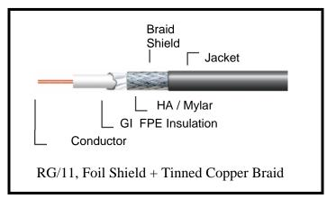
Belden and West Penn are the lead manufacturers of coaxial cable. Others make fine products, but the Belden and West Penn part numbers are usually used for base specifications and cross-referenced to other manufacturers.
