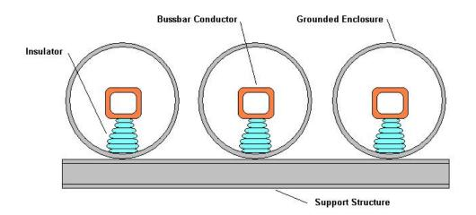
ISOLATED PHASE BUS DUCT CROSS SECTION DRAWING
