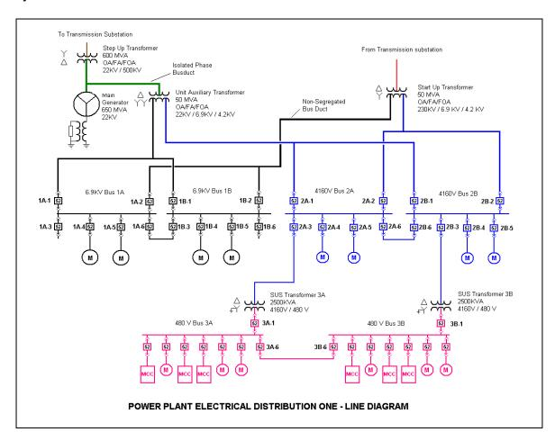
The one-line diagram shows a simplified arrangement of the primary electrical components. A more detailed discussion of each component follows this narrative.
