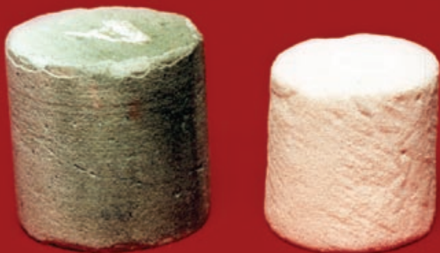
In the presence of CO 2 and hence carbonic acid, ThermoLock (left) remains unaffected for a long time, while Portland cement (right) quickly degrades.
